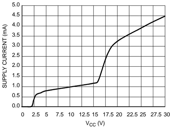
**Figure 9. Total Supply Current vs.  $V_{CC}$  (NCP346SN1)**
