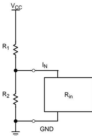
**Figure 4. Voltage divider input to adjust overvoltage detection point**
