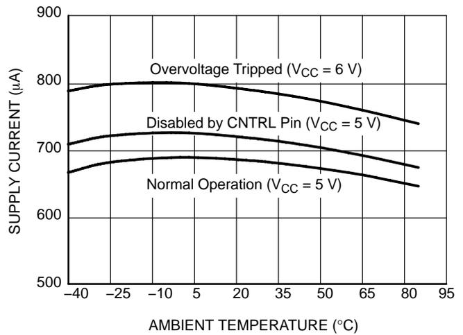
**Figure 8. Typical Supply Current ( $I_{CC} + I_{IN}$ ) vs. Temperature (NCP346SN2)**
