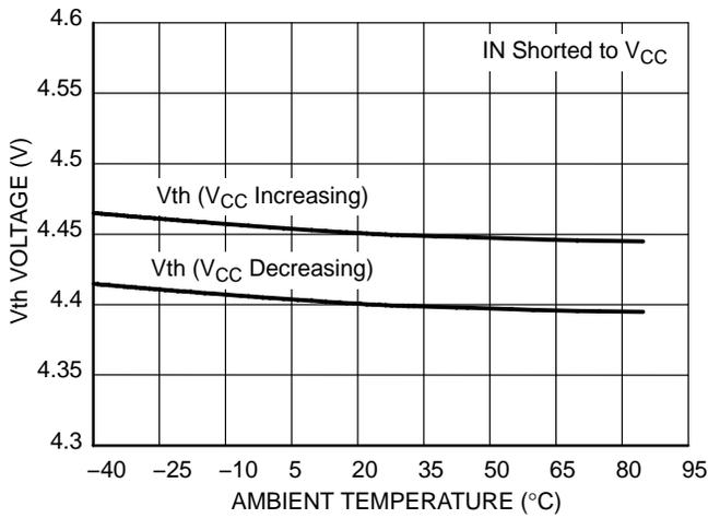
**Figure 5. Typical  $V_{th}$  Variation vs. Temperature (NCP346SN1)**
