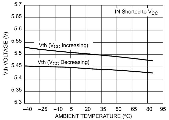
**Figure 6. Typical  $V_{th}$  Variation vs. Temperature (NCP346SN2)**
