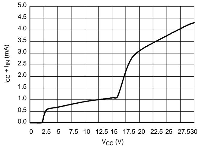
**Figure 10. Total Supply Current vs.  $V_{CC}$  (NCP346SN2)**
