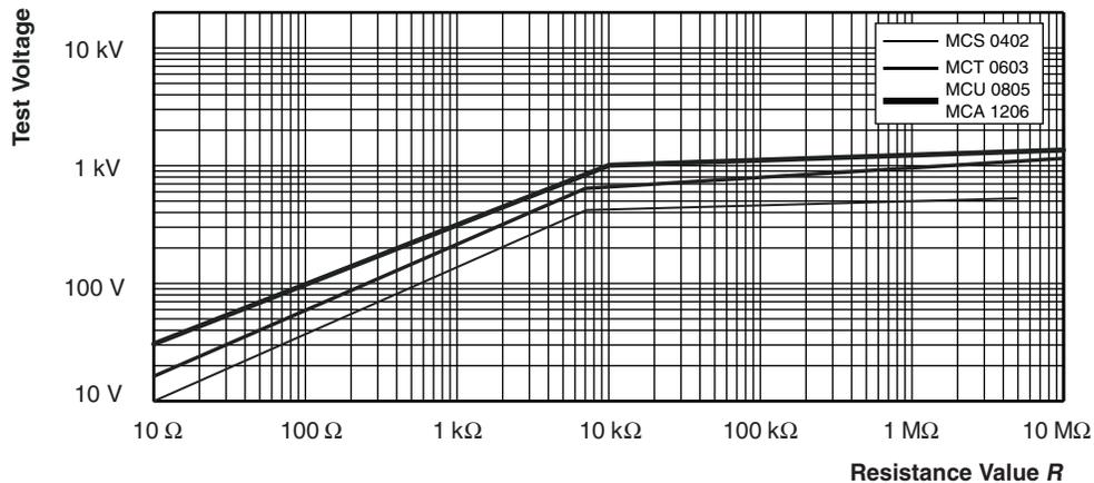
Pulse load rating in accordance with EN 60115-1 clause 4.27; 1.2  $\mu$ s/50  $\mu$ s; 5 pulses at 12 s interval;
