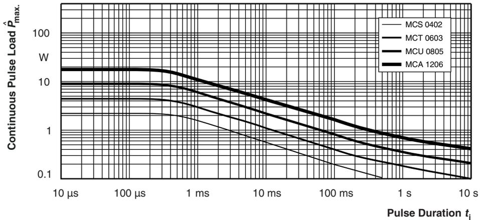
Maximum pulse load, continuous pulses; applicable if  $\bar{P} \leq P(\vartheta_{amb})$  and  $\hat{U} \leq \hat{U}_{max}$ ;
