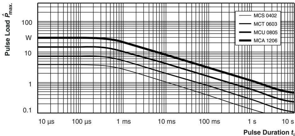
Maximum pulse load, single pulse; applicable if  $\bar{P} \rightarrow 0$  and  $n \leq 1000$  and  $\dot{U} \leq \dot{U}_{max}$ ;
