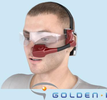
The FSM-9 can enable a wide range of hands-free controls on head mounted displays.
