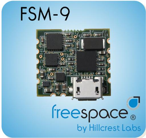
The FSM-9 is a low power, high performance motion tracking system which brings unprecedented motion realism to head mounted display (HMD), virtual reality, and augmented reality applications. The factory calibrated, tested, and optimized chip combines high performance MEMS sensors with MotionEngine™ Universal sensor fusion and cursor control software on a 32-bit MCU in a compact surface-mounted package.
