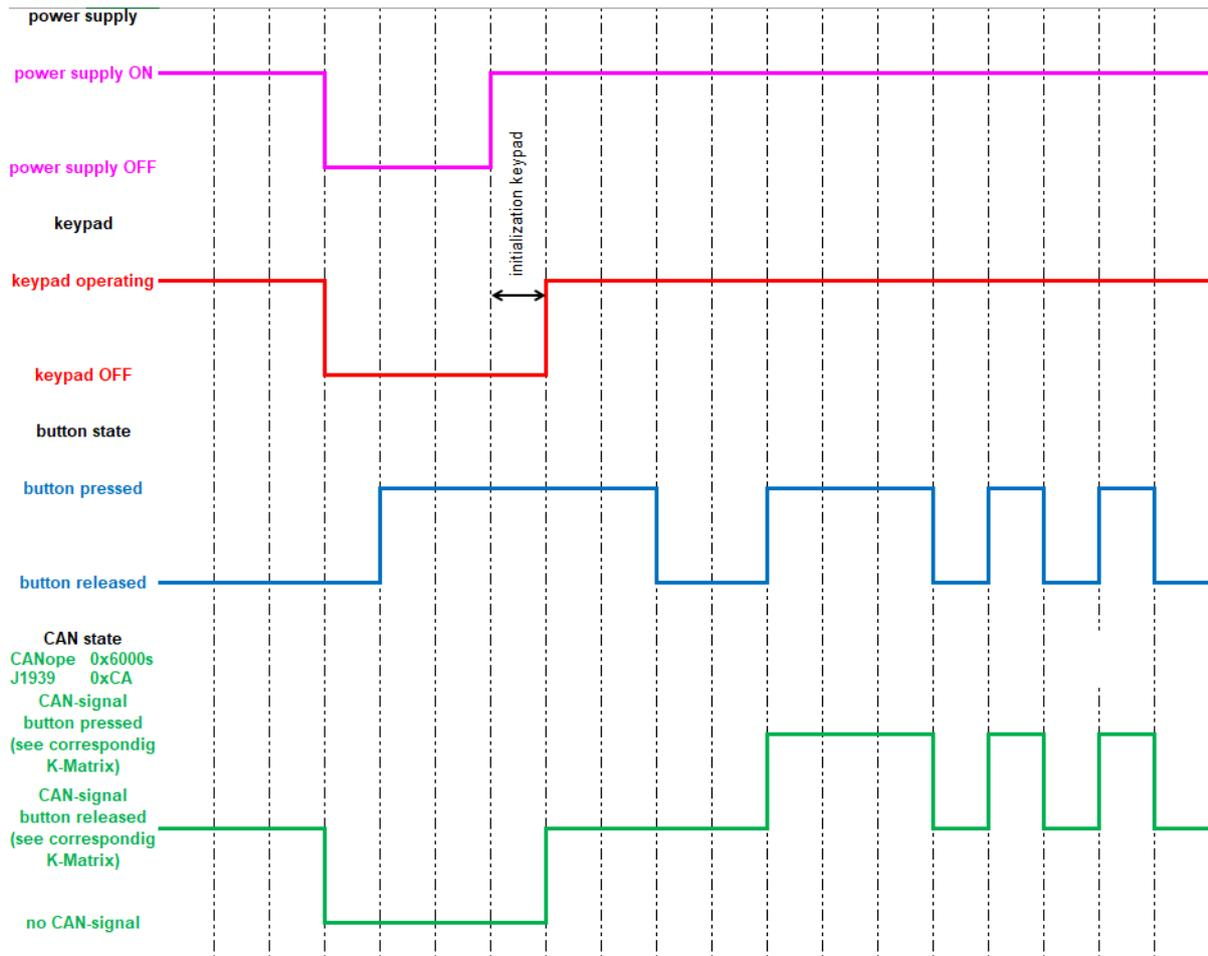
Picture 1: Button State after Power-On Reset
