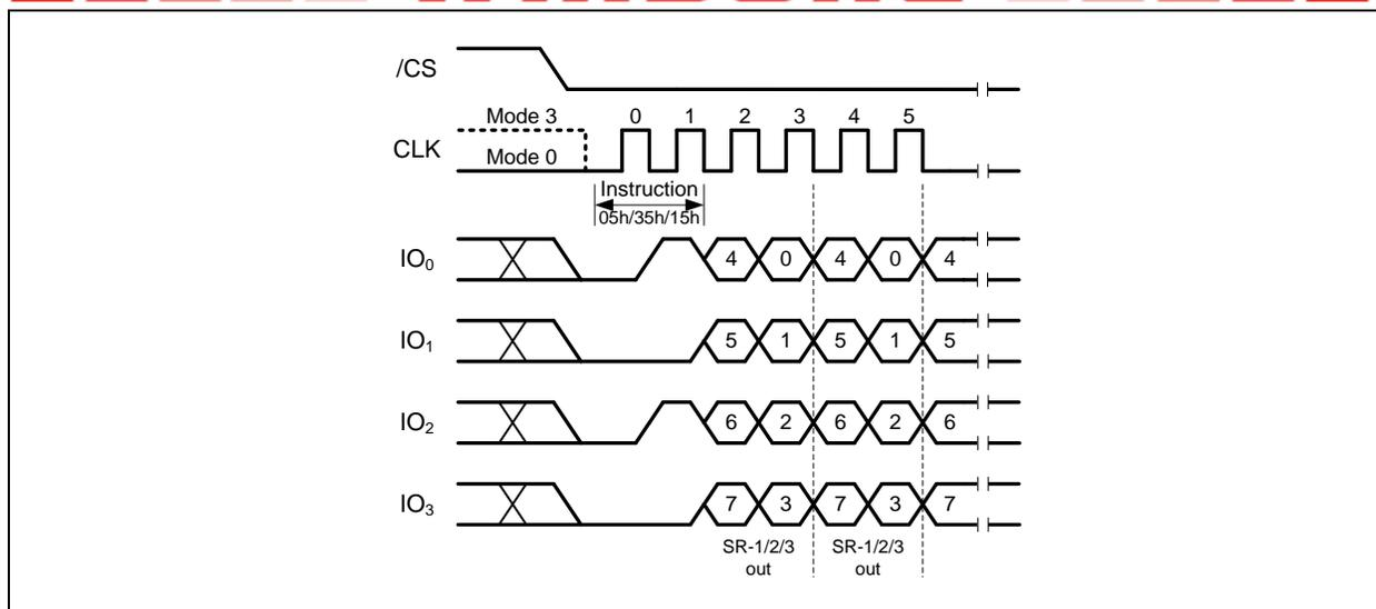
Figure 8b. Read Status Register Instruction (QPI Mode)
