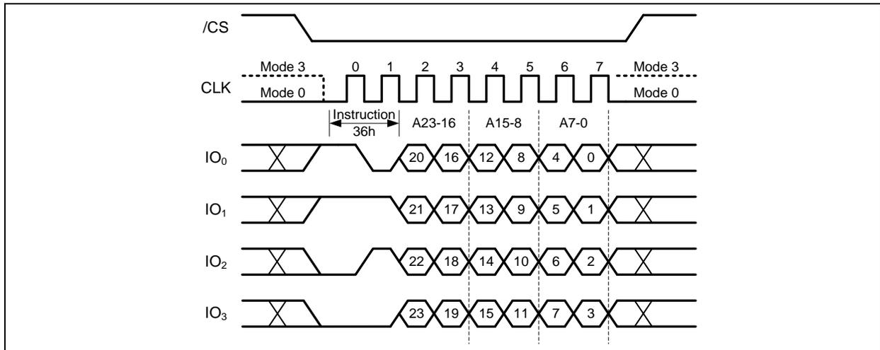
Figure 52b. Individual Block/Sector Lock Instruction (QPI Mode)
