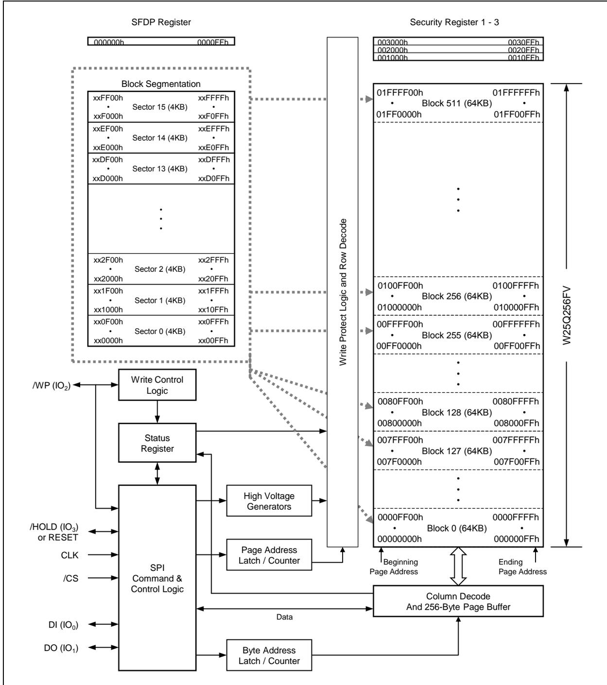
Figure 2. W25Q257FV Serial Flash Memory Block Diagram
