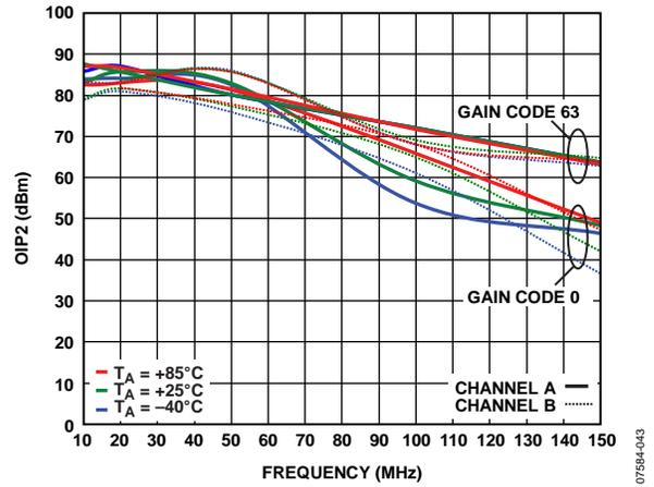
Figure 20. OIP2 vs. Frequency at Gain Code 0 and Gain Code 63, 2 V<sub>p-p</sub> Composite Output
