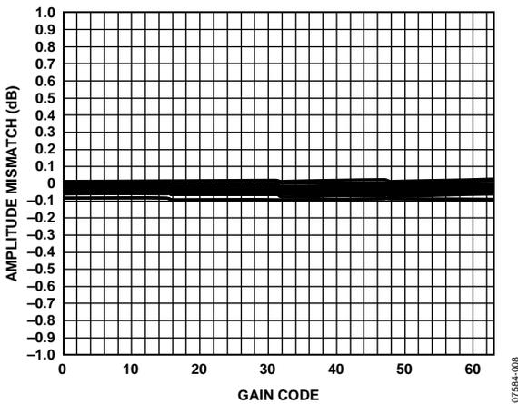
Figure 7. Channel A-to-Channel B Amplitude Mismatch vs. Gain Code, 2 V<sub>p-p</sub> Output
