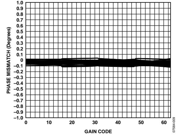
Figure 10. Channel A-to-Channel B Phase Mismatch vs. Gain Code, 2 V<sub>p-p</sub> Output
