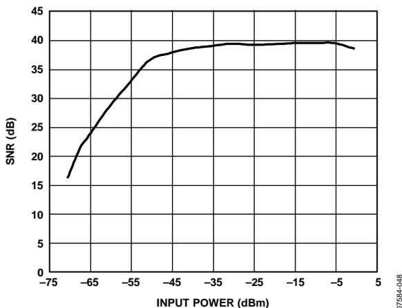
Figure 52. SNR vs. RF Input Power Level
