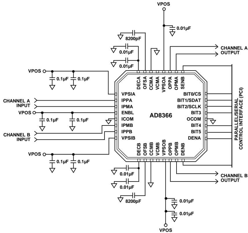
Figure 50. Basic Connections
