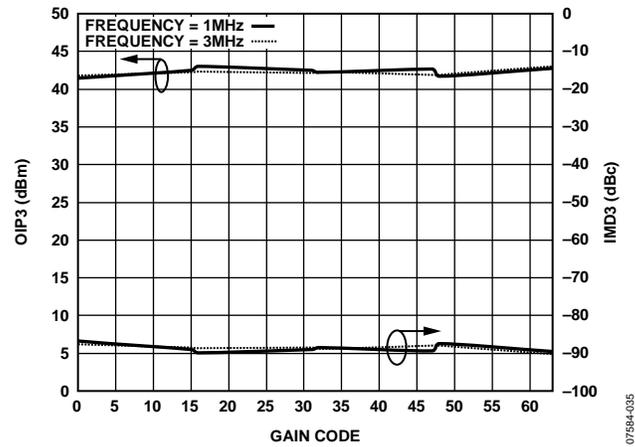
Figure 55. OIP3 on Low Frequency, 2 V p-p Composite
