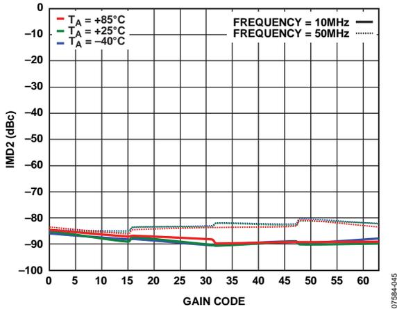
Figure 18. Two-Tone Output IMD2 vs. Gain Code at 10 MHz and 50 MHz Frequency, 2 V<sub>p-p</sub> Composite Output
