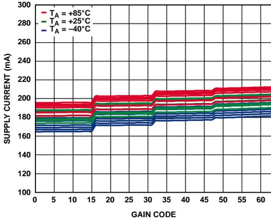
Figure 29. Supply Current vs. Gain Code at 10 MHz
