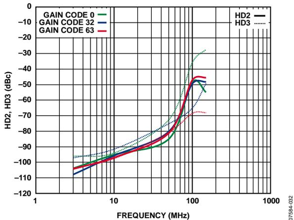
Figure 19. Harmonic Distortion vs. Frequency at Gain Code 0, Gain Code 32, and Gain Code 63, 2 V<sub>p-p</sub> Output
