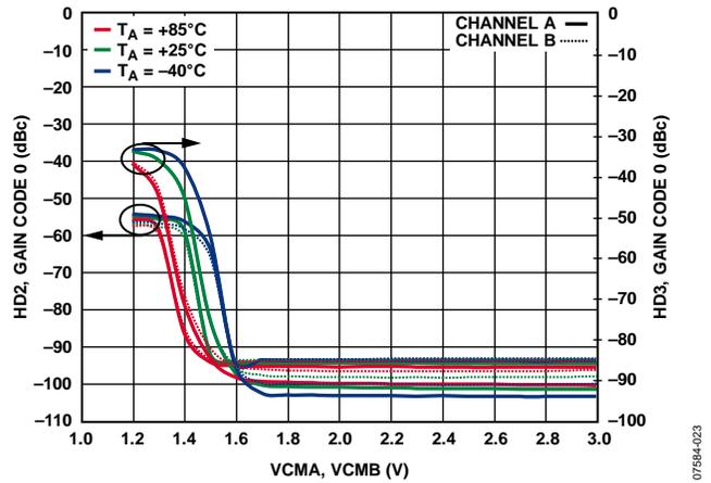
Figure 22. HD3/HD2 vs. V<sub>OCM</sub> at 10 MHz, Gain Code 0, 2 V<sub>p-p</sub> Output
