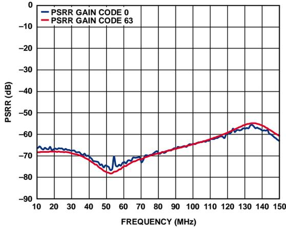
Figure 35. Power Supply Rejection Ratio (PSRR) vs. Frequency
