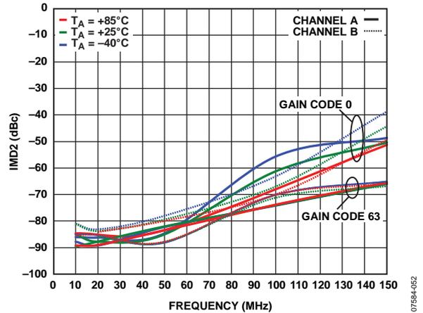
Figure 21. Two-Tone Output IMD2 vs. Frequency, Gain Code 0 and Gain Code 63, 2 V<sub>p-p</sub> Composite Output
