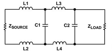
Figure 57. Schematic of a Fourth-Order, Chebyshev, Low-Pass Filter
