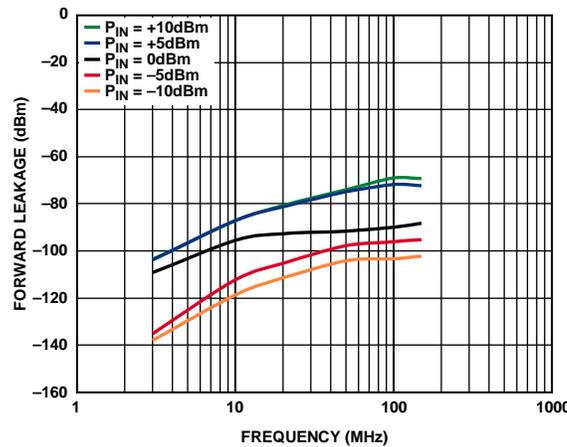
Figure 40. Forward Leakage vs. Frequency, Part Disabled
