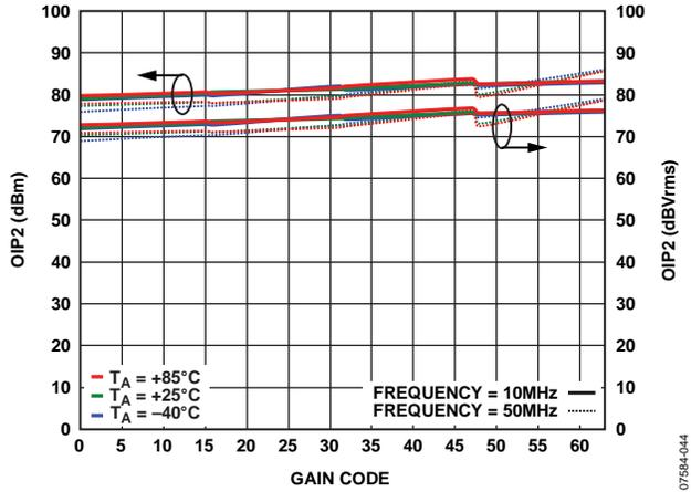
Figure 17. OIP2 vs. Gain Code at 10 MHz and 50 MHz Frequency, 2 V<sub>p-p</sub> Composite Output
