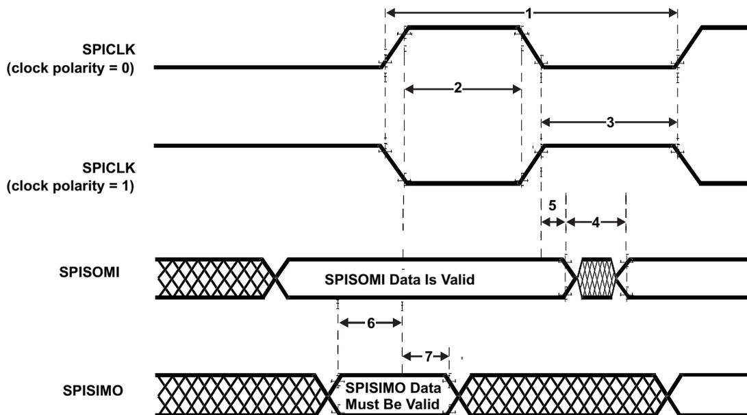
Figure 7-26. SPI Slave Mode External Timing (CLOCK PHASE = 1)
