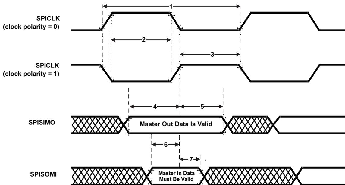
Figure 7-20. SPI Master Mode External Timing (CLOCK PHASE = 0)
