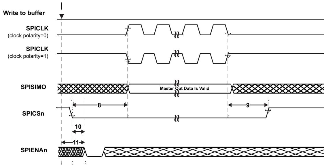
**Figure 7-23. SPI Master Mode Chip-Select Timing (CLOCK PHASE = 1)**
