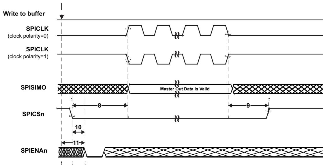
Figure 7-21. SPI Master Mode Chip-Select Timing (CLOCK PHASE = 0)
