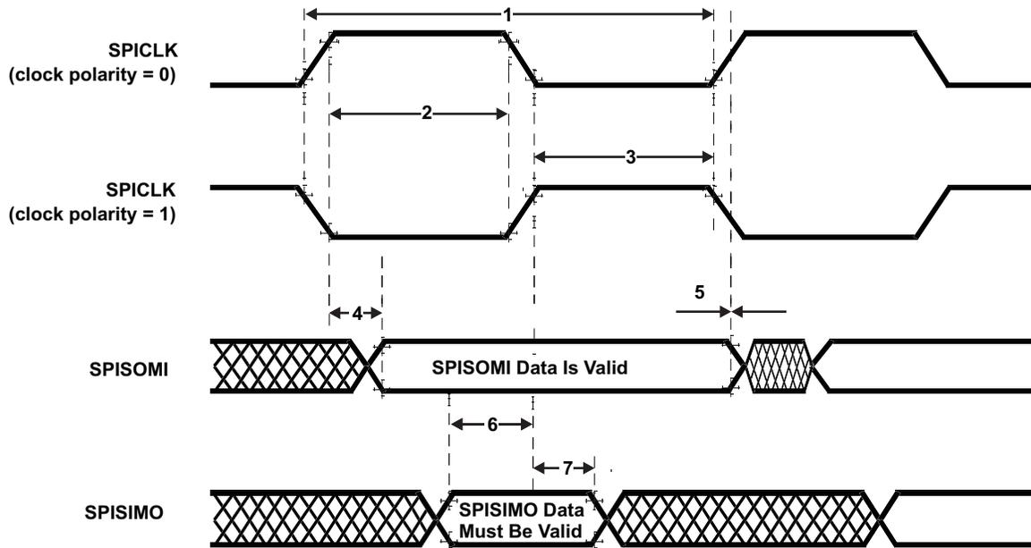
Figure 7-24. SPI Slave Mode External Timing (CLOCK PHASE = 0)
