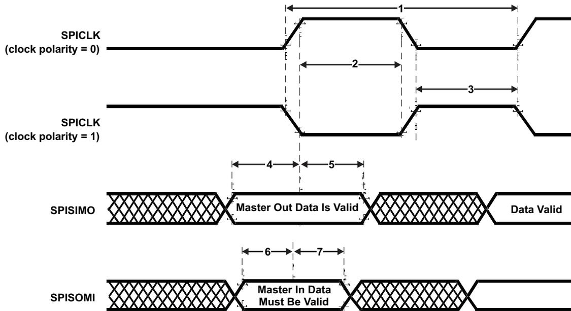
**Figure 7-22. SPI Master Mode External Timing (CLOCK PHASE = 1)**
