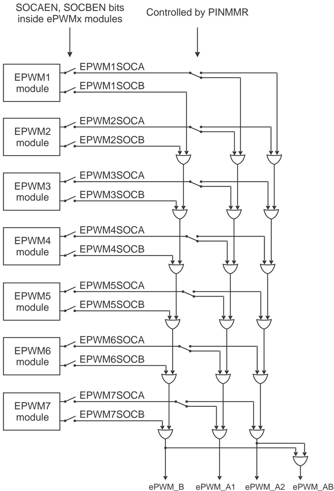
Figure 7-10. ADC Trigger Source Generation from ePWMx
