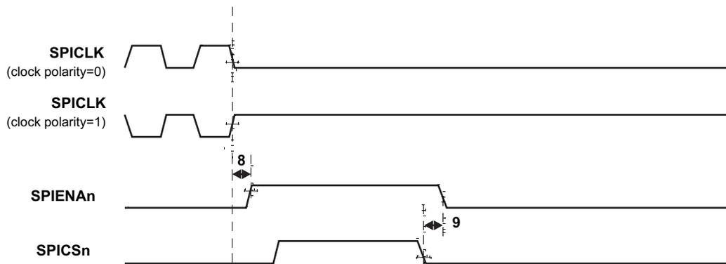
Figure 7-25. SPI Slave Mode Enable Timing (CLOCK PHASE = 0)
