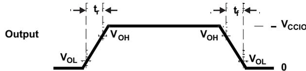
**Figure 7-2. CMOS-Level Outputs**
