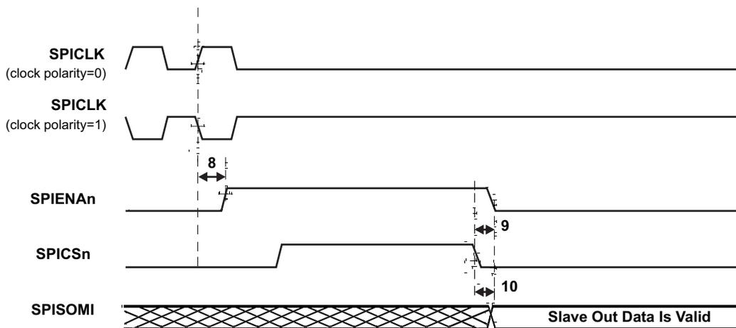
Figure 7-27. SPI Slave Mode Enable Timing (CLOCK PHASE = 1)
