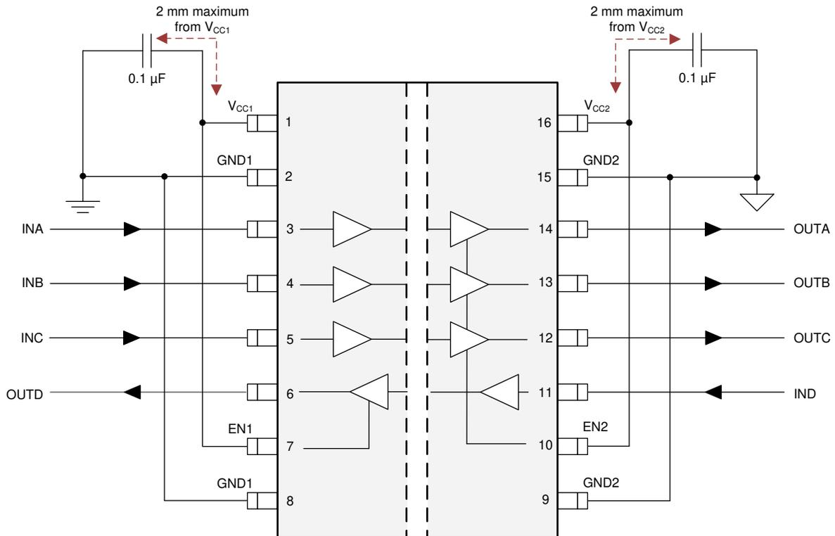
**Figure 10-2. Typical ISOS141-SEP Circuit Hook-up**
