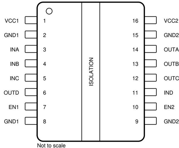
**Figure 5-1. ISOS141-SEP DBQ Package 16-pin QSOP Top View**
