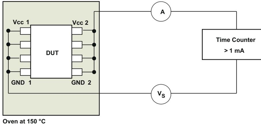
**Figure 10-6. Test Setup for Insulation Lifetime Measurement**
