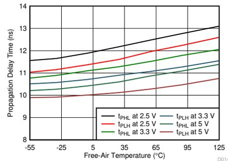
**Figure 6-8. Propagation Delay Time vs Free-Air Temperature**
