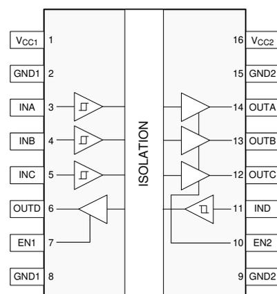
V<sub>CC1</sub>=Input supply, V<sub>CC2</sub>=Output supply
