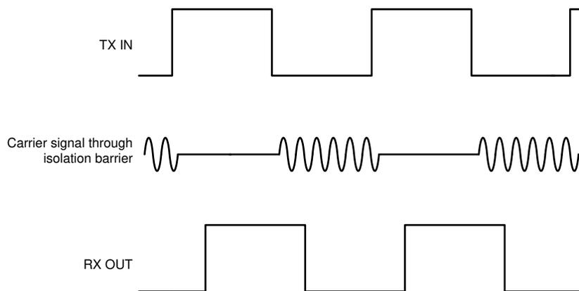
**Figure 9-2. On-Off Keying (OOK) Based Modulation Scheme**
