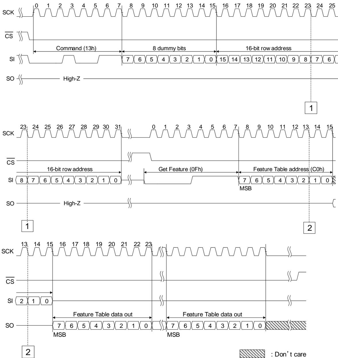
Figure 11. Page Read from Cell Array to Buffer
