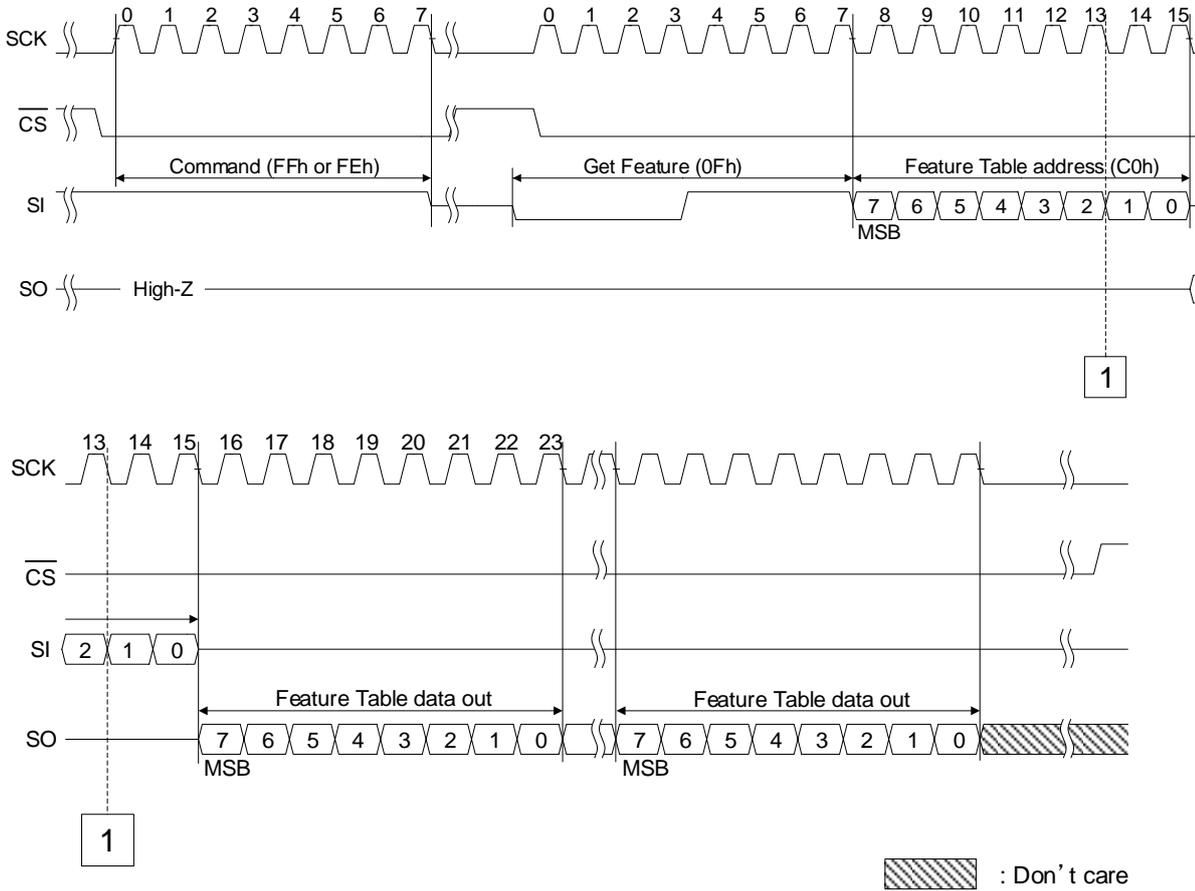
Figure 19. Reset Timing
