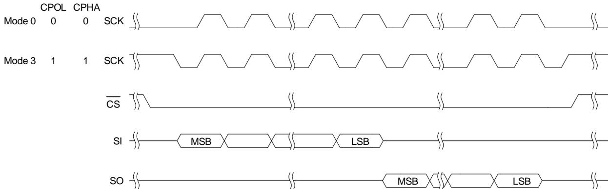
Figure 5. SPI Timing
