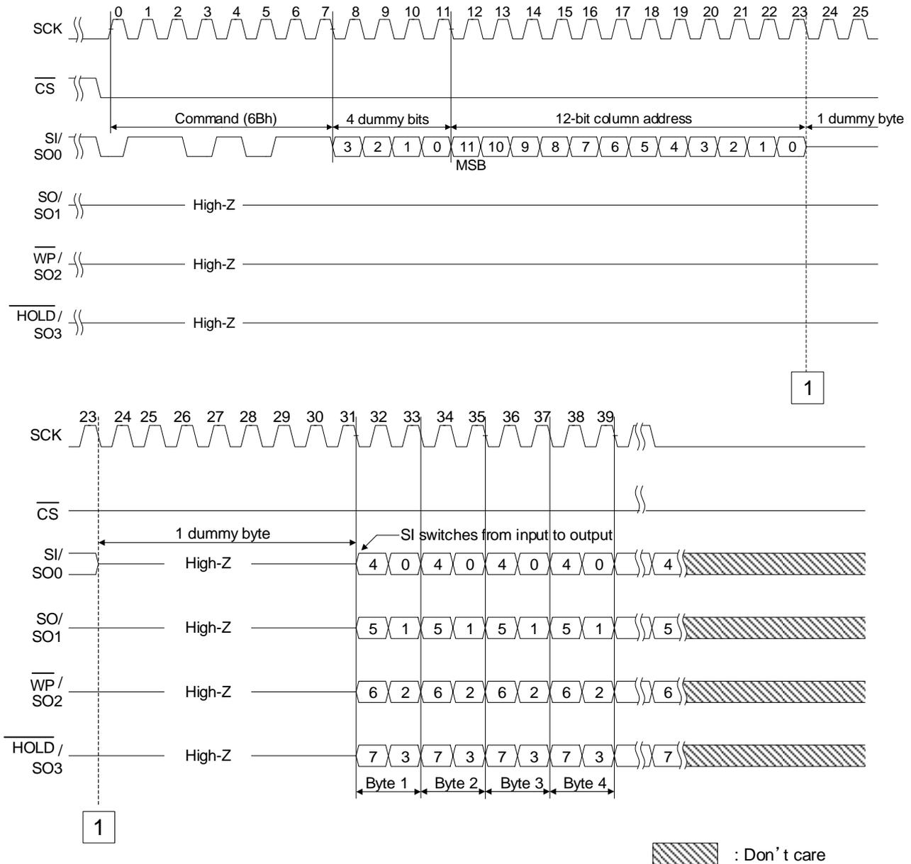
Figure 14. Page Read from Buffer x4 Timing
