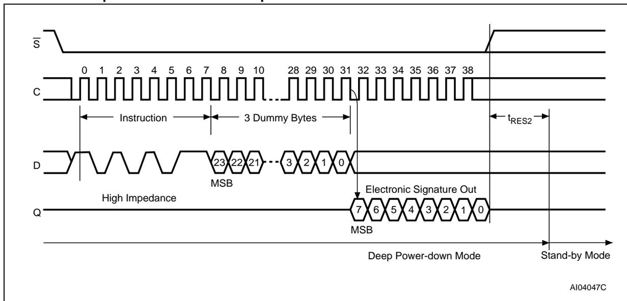
1. The value of the 8-bit Electronic Signature, for the M25P40, is 12h.
