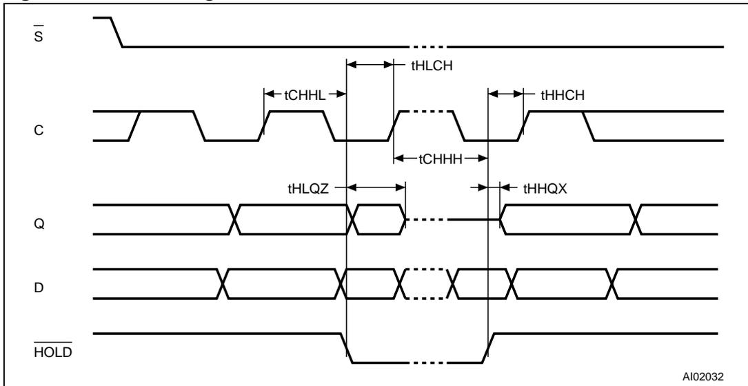
Figure 25. Output Timing
