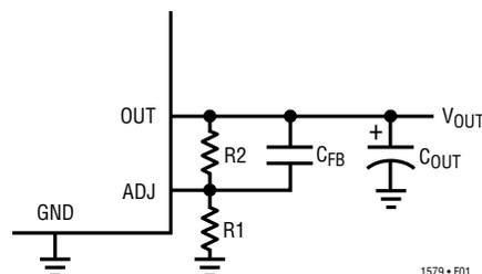
Figure 1. Adjustable Operation
