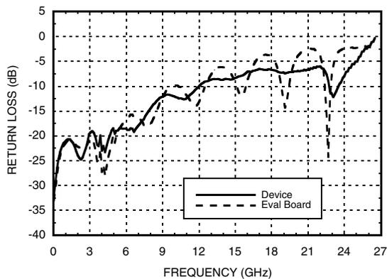
[1] VR = 0.0 V      [2] Frequency = 32 Gbps      [3] Device measured on evaluation board with gating after connector
