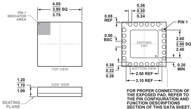
24-Terminal Ceramic Leadless Chip Carrier [LCC]
