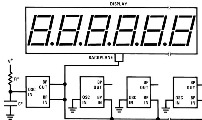
\*The minimum recommended value for R for the oscillator input is 9 k $\Omega$ . An RC time constant of approximately  $4.91 \times 10^{-4}$  should produce a backplane frequency between 30 Hz and 150 Hz.
