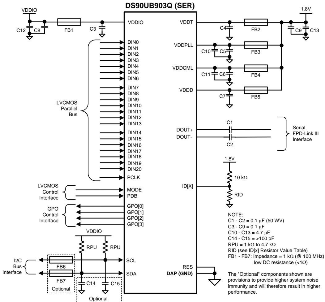
Figure 37. DS90UB903Q Typical Connection Diagram — Pin Control
