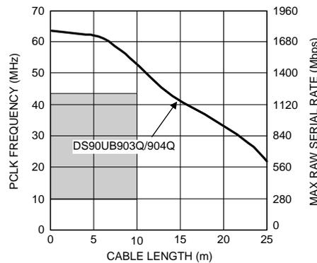
\*Note: Equalization is enabled for cable lengths greater than 7 meters
