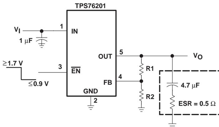
**Figure 18. TPS76201 Adjustable LDO Regulator Programming**
