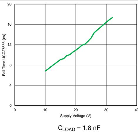
Figure 6. UCC27536 Fall Time vs. Supply Voltage
