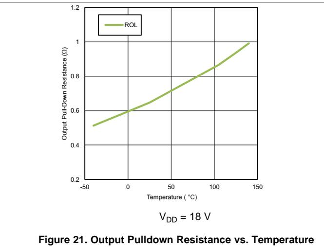
Figure 21. Output Pulldown Resistance vs. Temperature
