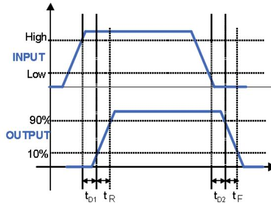
Figure 1. UCC27531: (Output = OUTH Tied to OUTL) Input = IN, (EN = VDD), or Input = EN, (IN = VDD)
