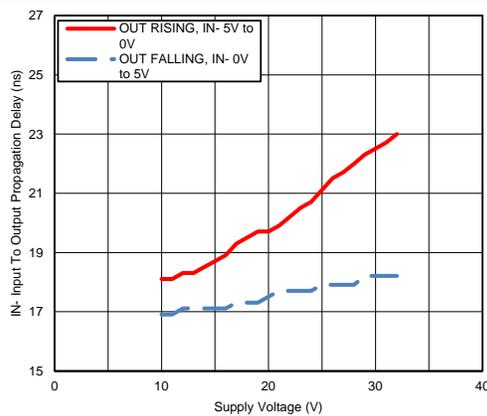
Figure 8. IN- Propagation Delay vs. Supply
