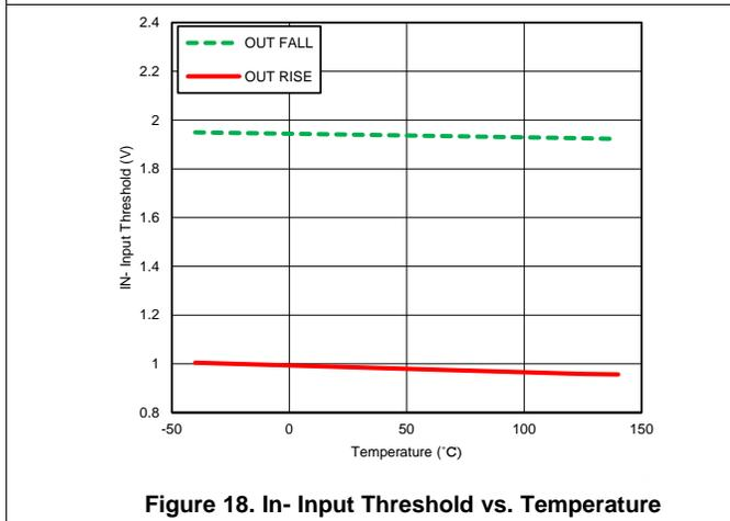
Figure 18. In- Input Threshold vs. Temperature
