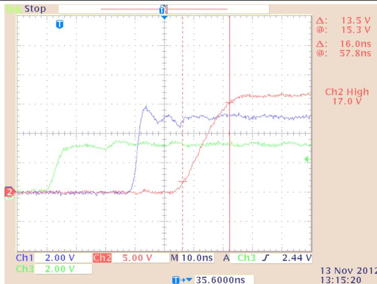
Figure 44. UCC27531DBV Input vs. Output PWM Rise Time
