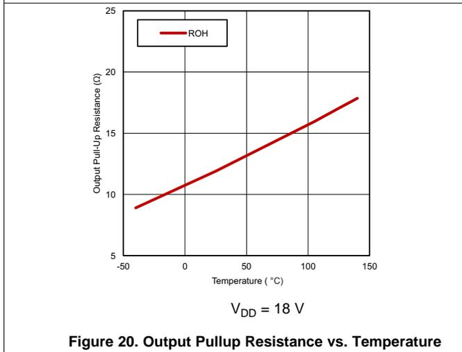
Figure 20. Output Pullup Resistance vs. Temperature
