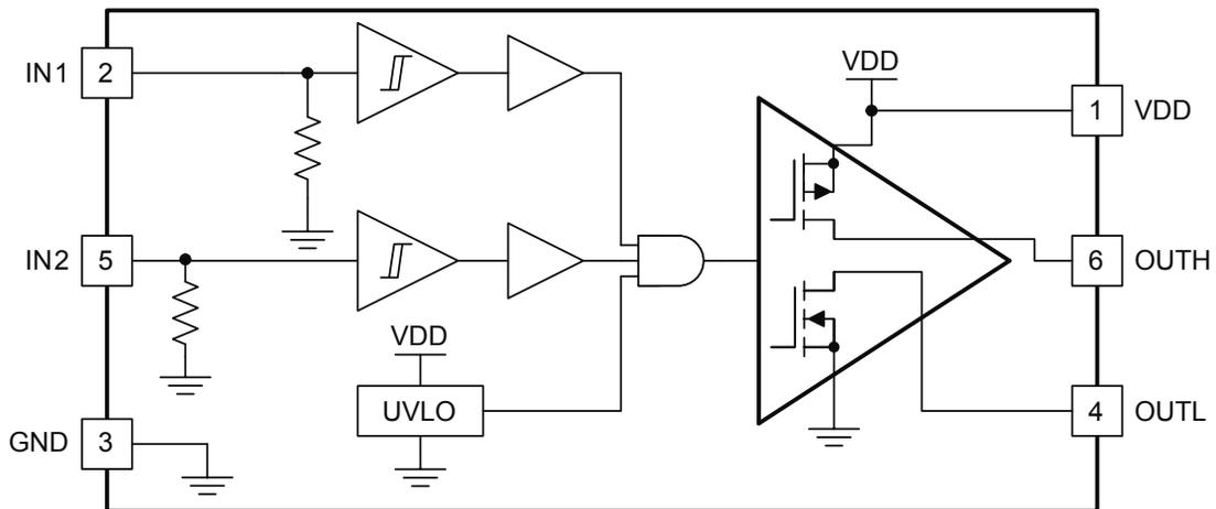
IN1 Pull-Down Resistance to GND = 230 kΩ, IN2 Pull-Down Resistance to GND = 230 kΩ
