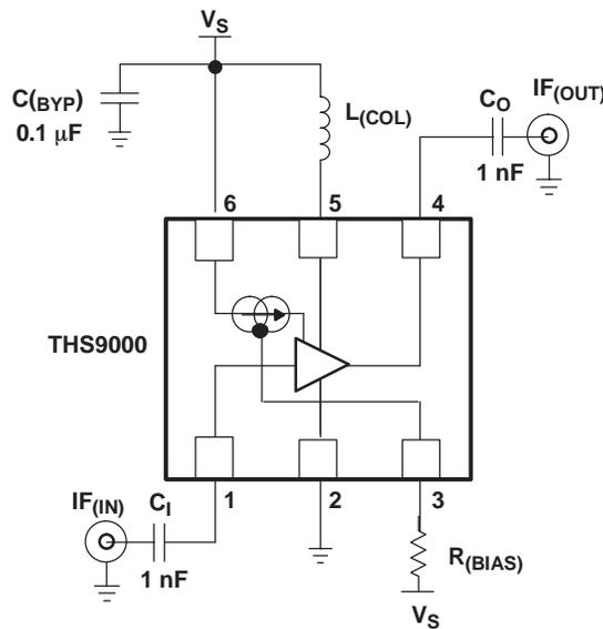
Figure 26. THS9000 Recommended Circuit (used for all tests)
