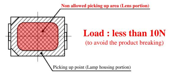
Please adjust the load, the pick up point, the nozzle diameter, etc. before mounting because the over load can cause the breakage of the lamp housing.
