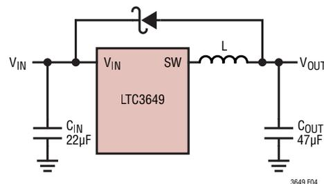
Figure 4. Schottky Diode from  $V_{OUT}$  to  $V_{IN}$
