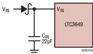
Figure 3. Schottky Diode in Series with the Supply
