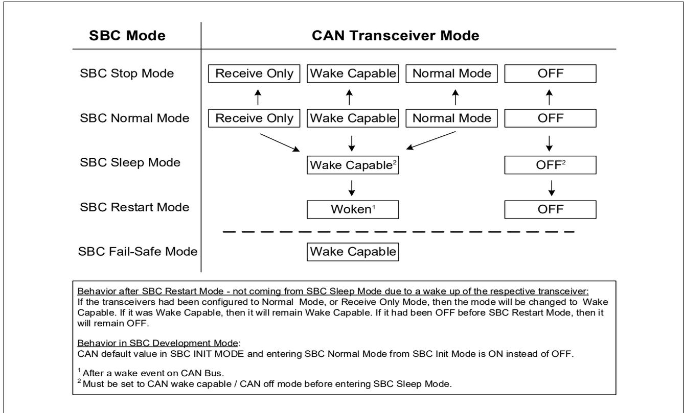
Figure 26 CAN Mode Control Diagram
