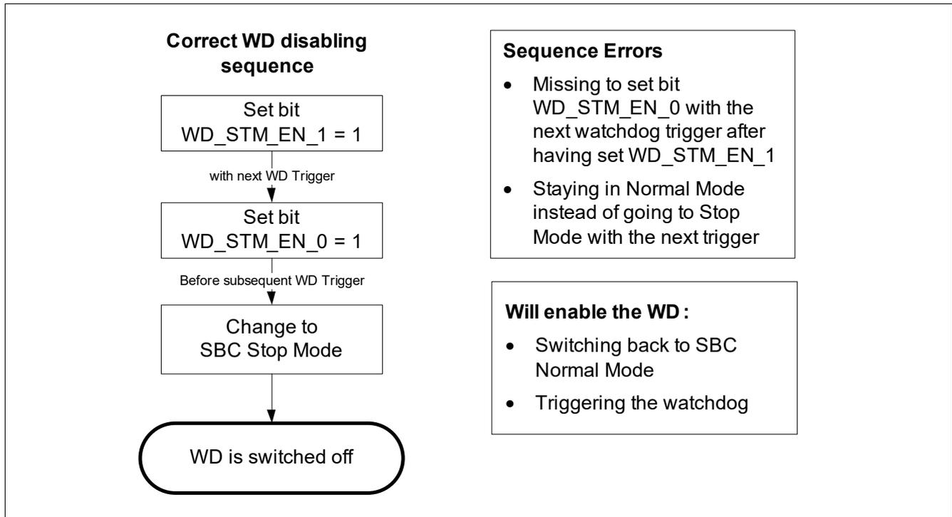
**Figure 50** Watchdog disabling sequence in SBC Stop Mode
