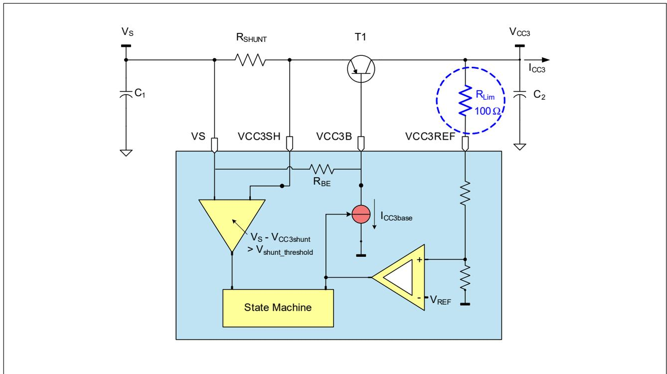
**Figure 19** Protecting the VCC3 against inductive short circuits when configured as an independent voltage regulator for off-board supply
