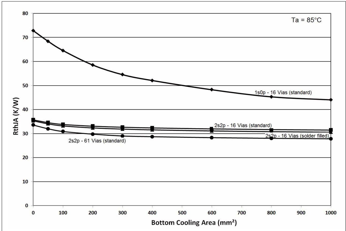
Figure 62 Thermal Resistance ( $R_{th\_JA}$ ) vs. Cooling Area
