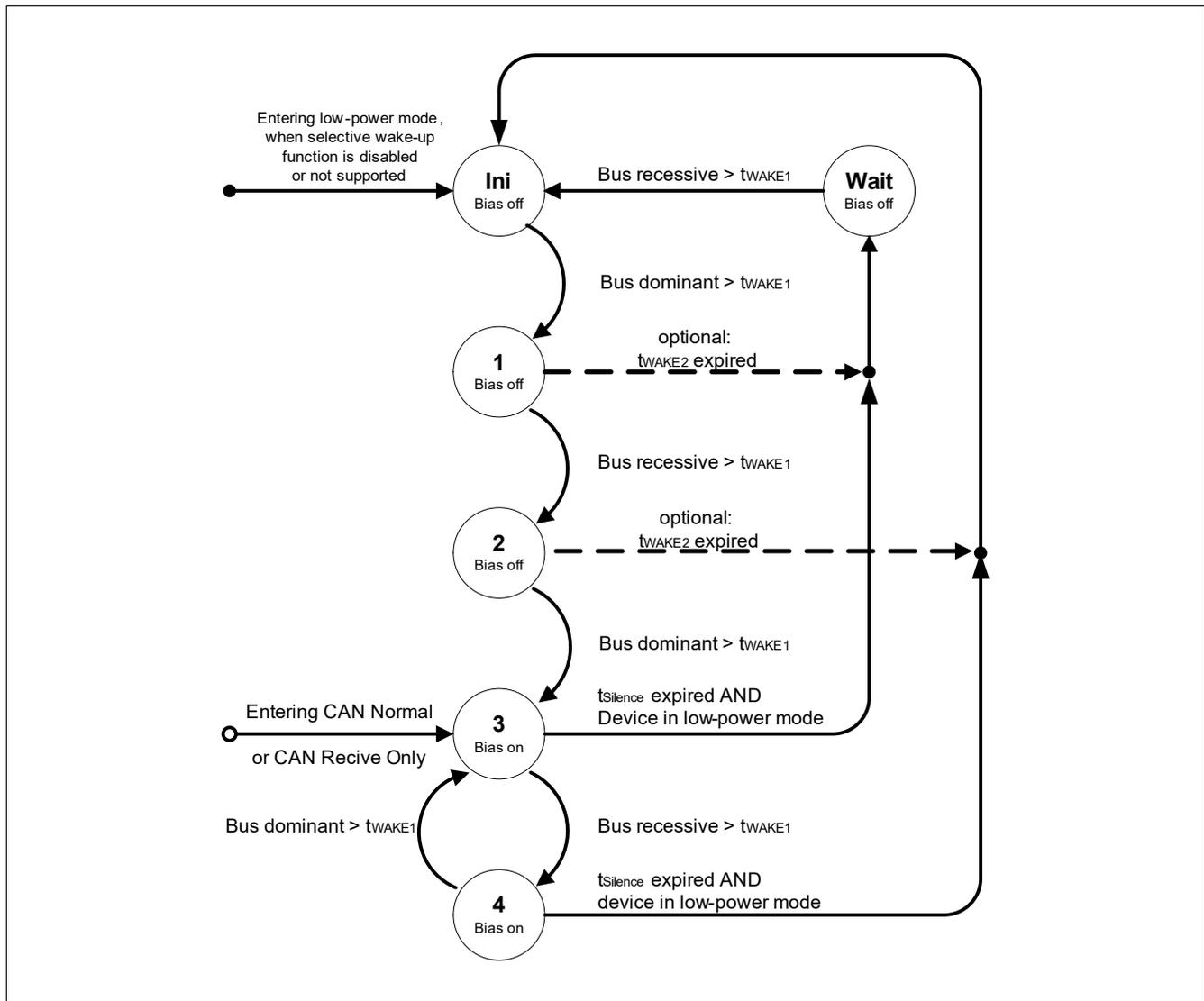
**Figure 29 WUP detection following the definition in ISO 11898-2:2016**
