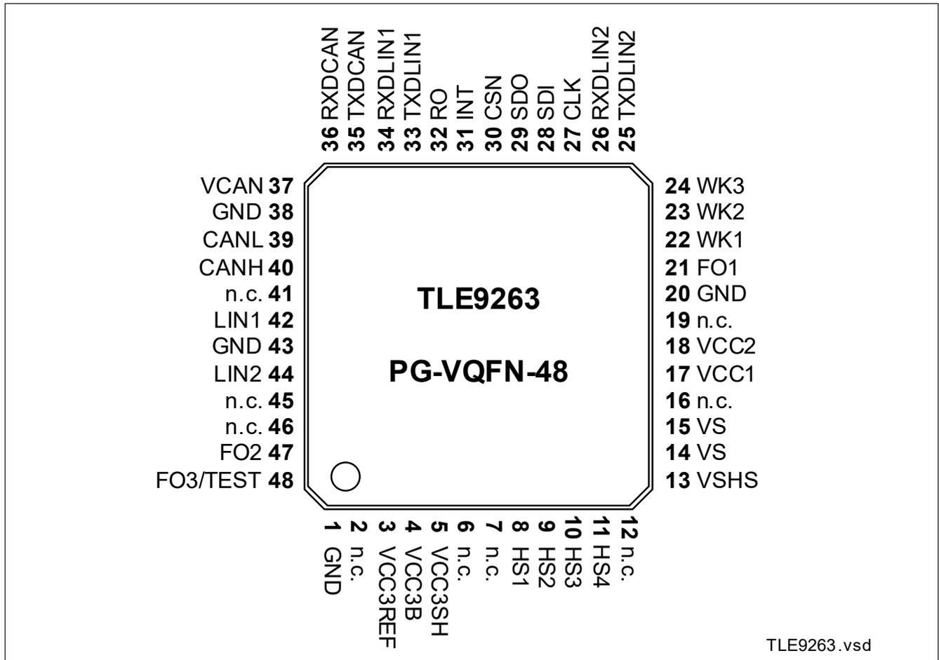
Figure 2 Pin Configuration
