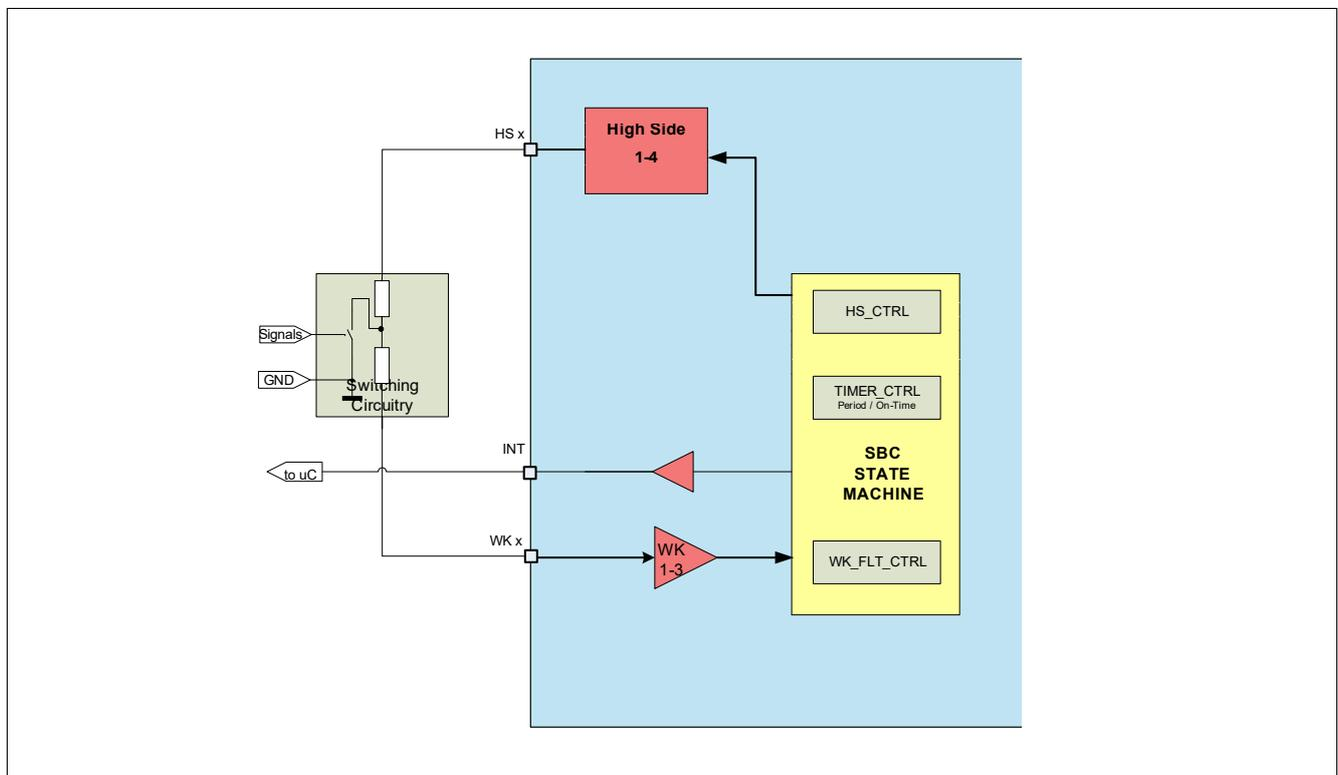
**Figure 5** Cyclic Sense Working Principle
