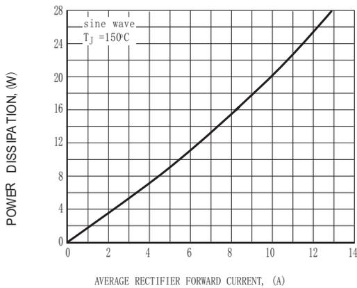
FIG. 3 FORWARD DISSIPATION
