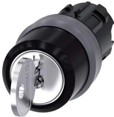
RONIS key-operated switch, 22 mm, round, plastic with metal front ring, lock number SB30, with 2 keys, 3 switch positions I-O<II, left latching, right momentary contact type, actuating angle 2x45°, 10:30h/12h/13:30h, key removal O, possible special locks: SB31, 421, 455, with laser labeling, upper case and lower case, always upper case at beginning of line
