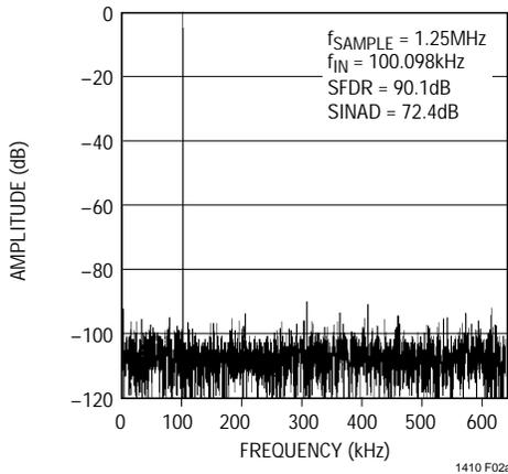
Figure 2a. LTC1410 Nonaveraged 4096 Point FFT, 100kHz Input
