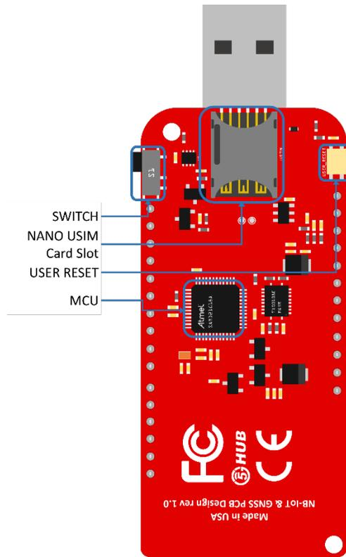
Figure 5. USB Dongle Bottom Side – Key Components
