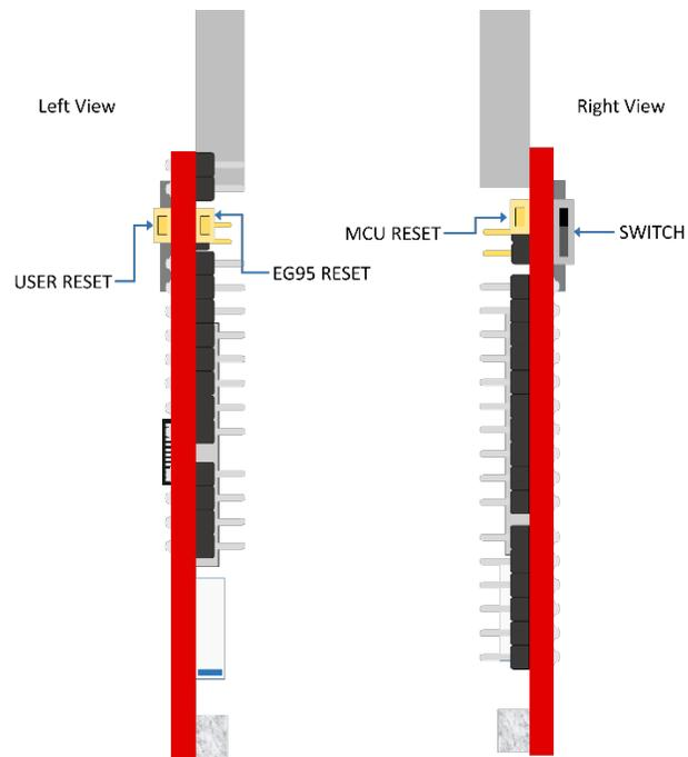
Figure 6. USB Dongle Side View – Key Components
