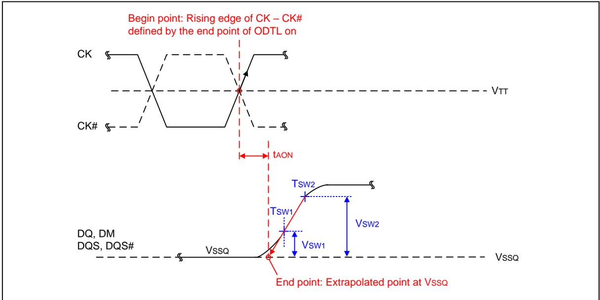
Figure 99 – Definition of t<sub>AON</sub>
