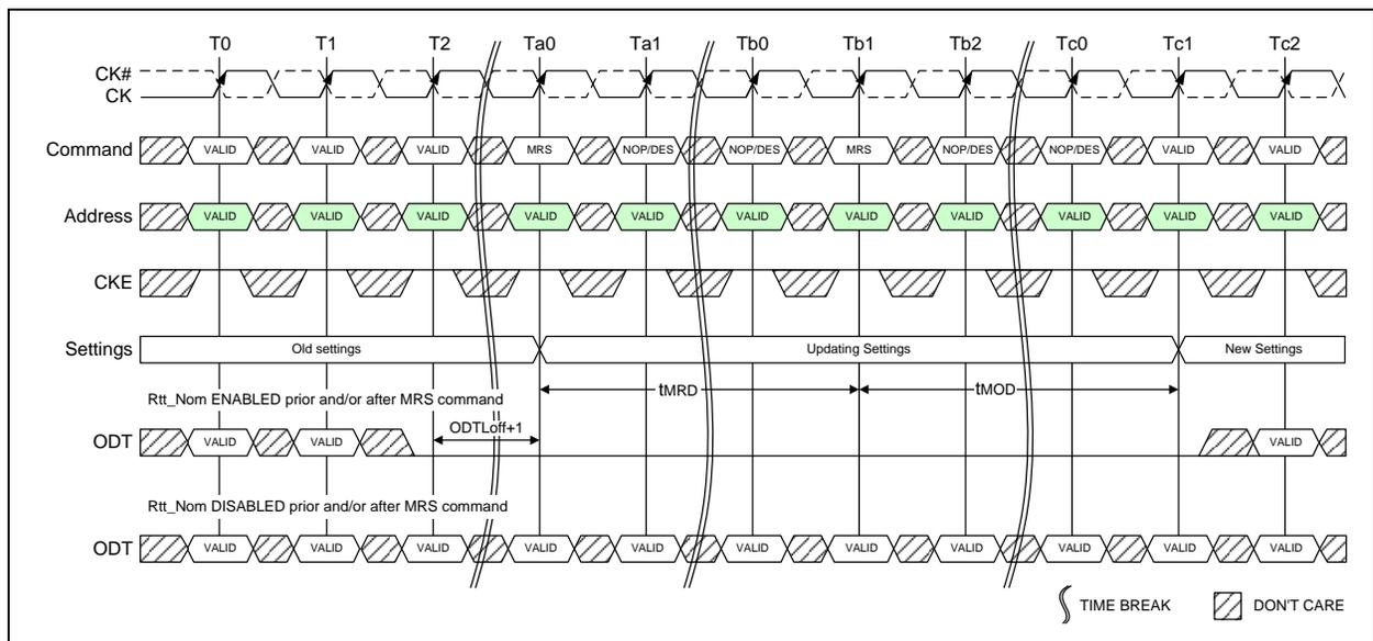
Figure 3 – tMRD Timing
