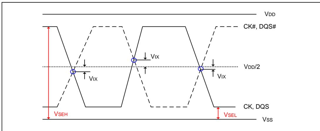
**Figure 92 –  $V_{IX}$  Definition**
