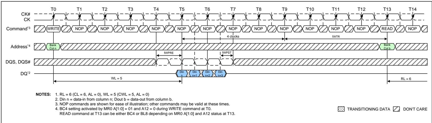
Figure 51 – WRITE (BC4) to READ (BC4) OTF
