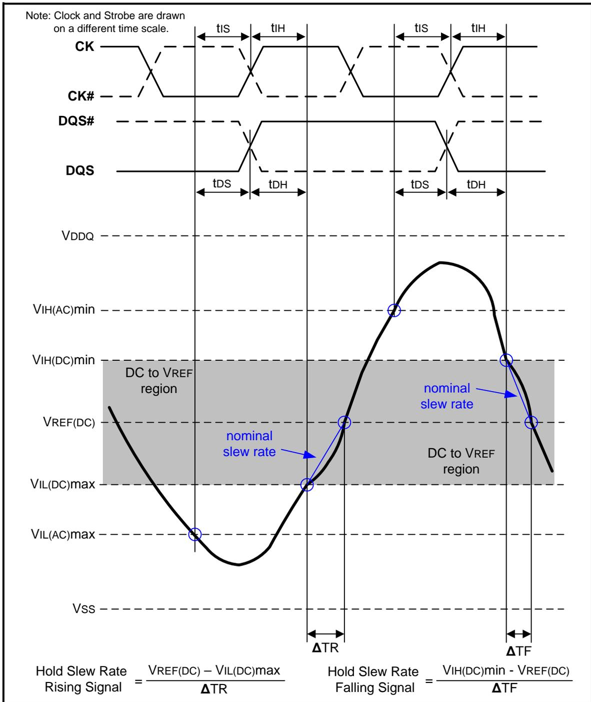
Figure 108 – Illustration of nominal slew rate for hold time t<sub>DH</sub> (for DQ with respect to strobe) and t<sub>IH</sub> (for ADD/CMD with respect to clock)
