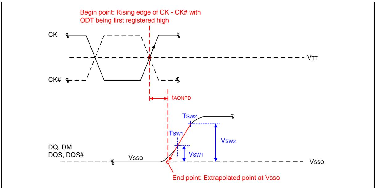
Figure 100 – Definition of t<sub>AONPD</sub>
