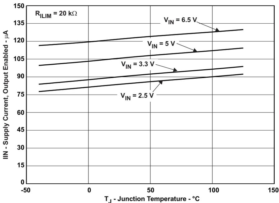
Figure 18.  $I_{IN}$  – Supply Current, Output Enabled –  $\mu A$
