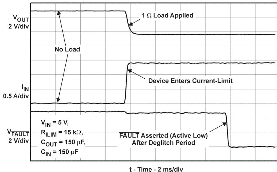
Figure 12. No Load to 1 $\Omega$  Transient Response
