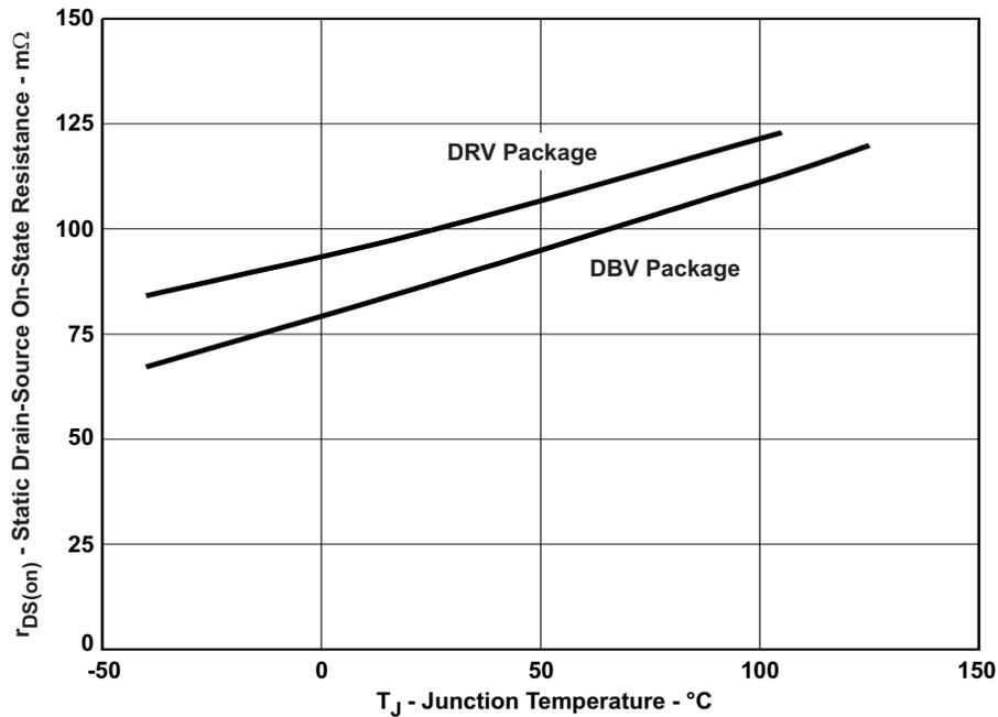
Figure 20. MOSFET r<sub>DS(on)</sub> Vs. Junction Temperature
