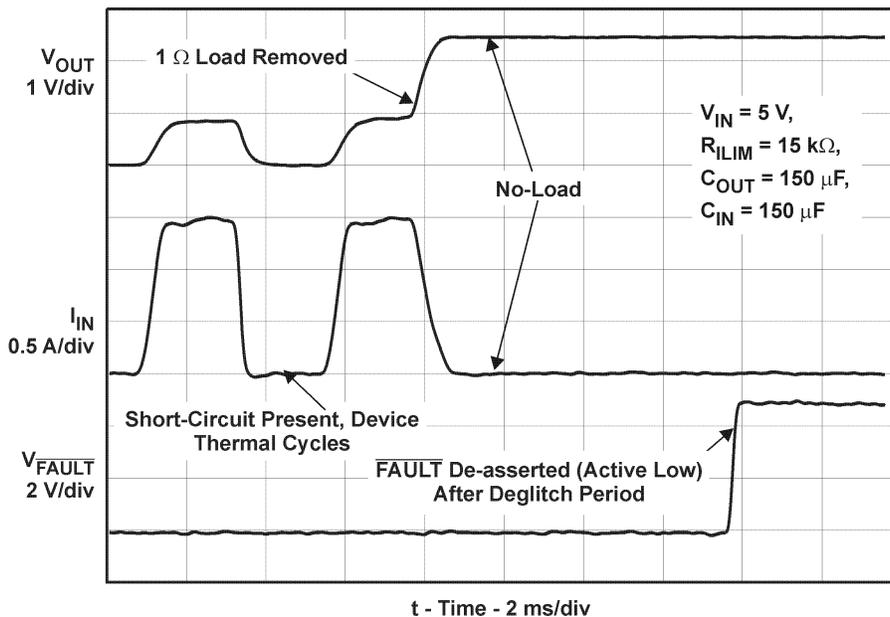
Figure 13. 1Ω to No Load Transient Response
