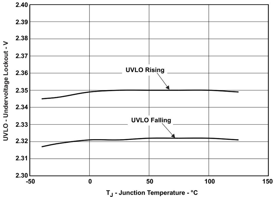
Figure 16. UVLO – Undervoltage Lockout – V
