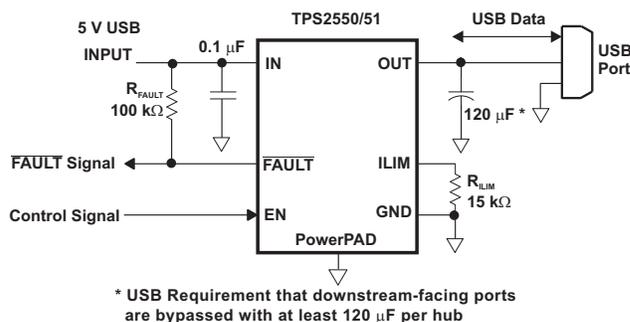
\* USB Requirement that downstream-facing ports are bypassed with at least 120  $\mu$ F per hub
