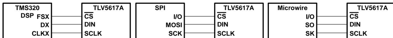
Figure 12. Three-Wire Interface
