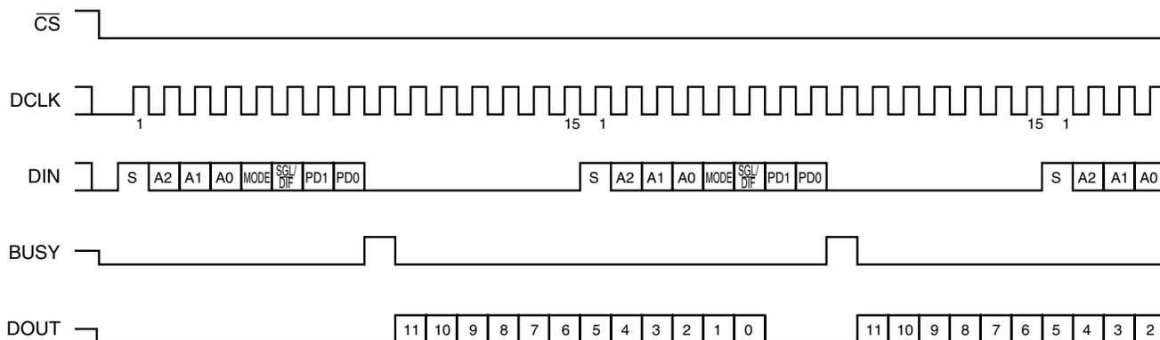
Figure 6. Maximum Conversion Rate, 15 Clock Cycles Per Conversion
