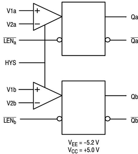
**Figure 2. Logic Diagram**
