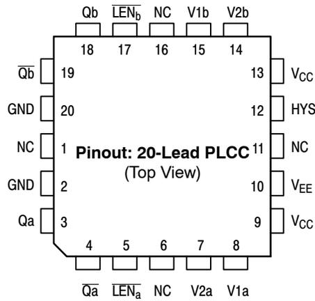
\* All V<sub>CC</sub> and V<sub>CCO</sub> pins are NOT tied together on the die.
