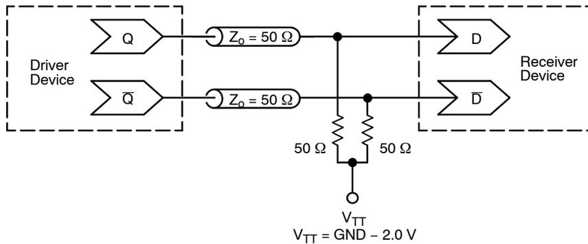
**Figure 8. Typical Termination for Output Driver and Device Evaluation**
