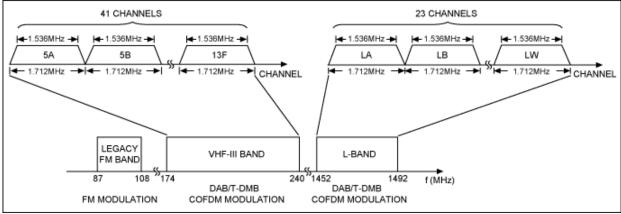
Figure 2. DAB RF signal frequency plan.
