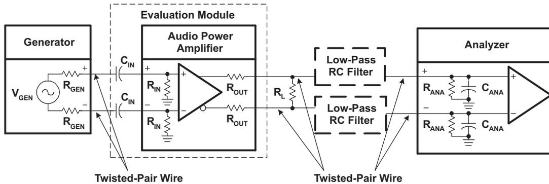
Figure 29. Differential Input, BTL Output Measurement Circuit
