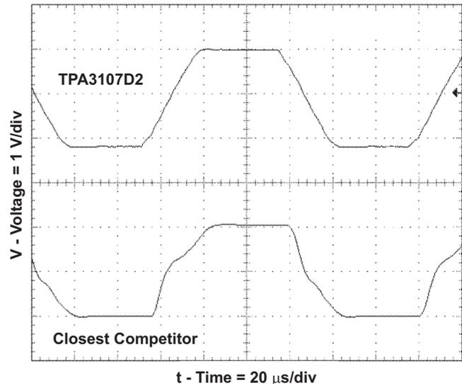
Figure 26. 8-kHz Sine Output at 10% THD+N
