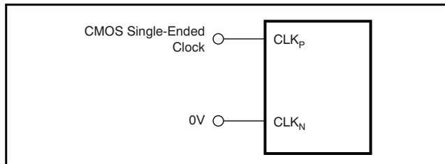
**Figure 35. Single-Ended Clock Driving Circuit (DIFF\_CLK = 0)**
