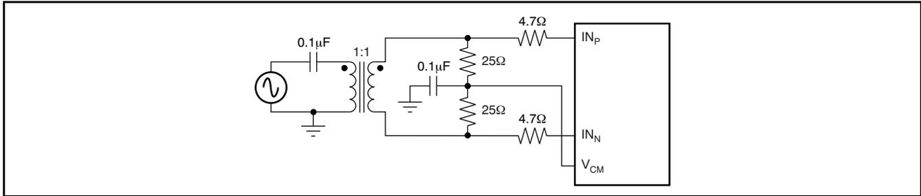
Figure 33. Drive Circuit at Low Input Frequencies
