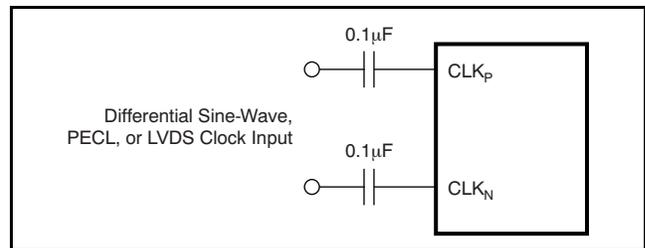
**Figure 37. Differential Clock Driving Circuit (DIFF\_CLK = 1)**
