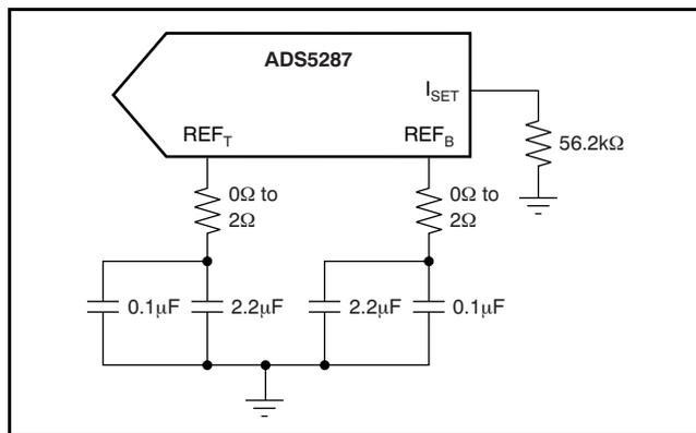
Figure 40. Suggested Decoupling on the Reference Pins
