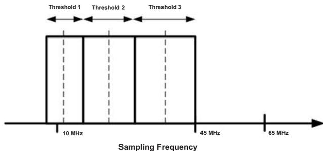
**Figure 39. Variation of Thresholds Across Sampling Frequency**
