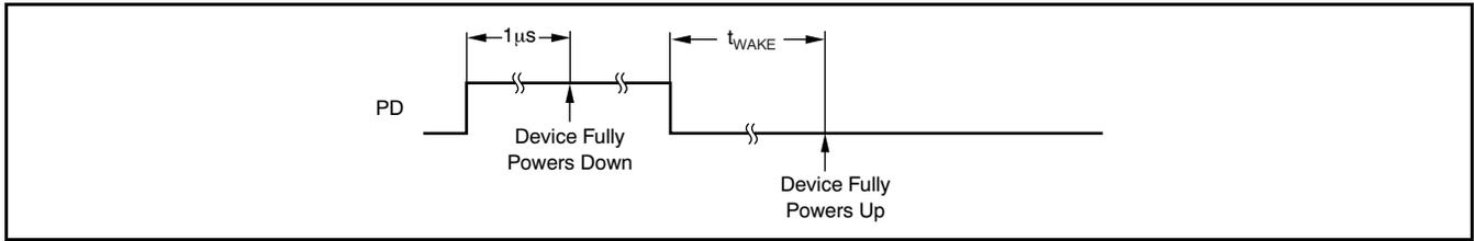
Power-up time shown is based on 1 μF bypass capacitors on the reference pins. t<sub>WAKE</sub> is the time it takes for the device to wake up completely from power-down mode. The ADS5287 has two power-down modes: complete power-down mode and partial power-down mode. The device can be configured in partial power-down mode through a register setting.
