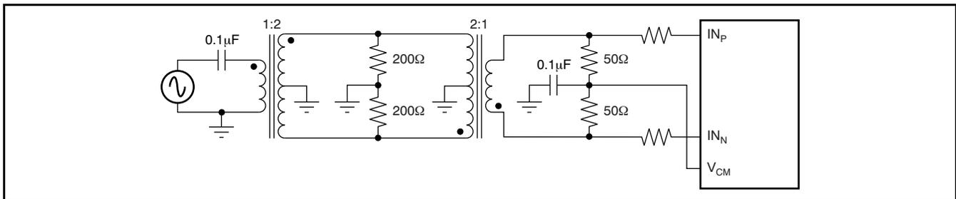
Figure 34. Drive Circuit at High Input Frequencies
