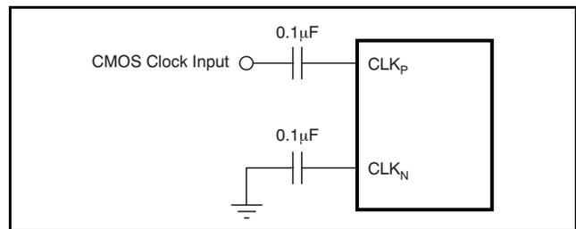
**Figure 38. Single-Ended Clock Driving Circuit When DIFF\_CLK = 1**
