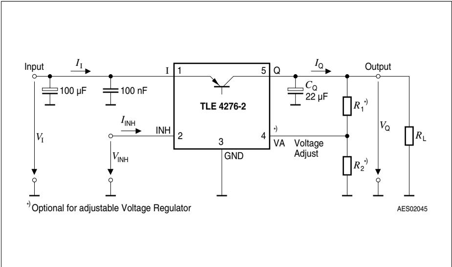
**Figure 3 Measuring Circuit**
