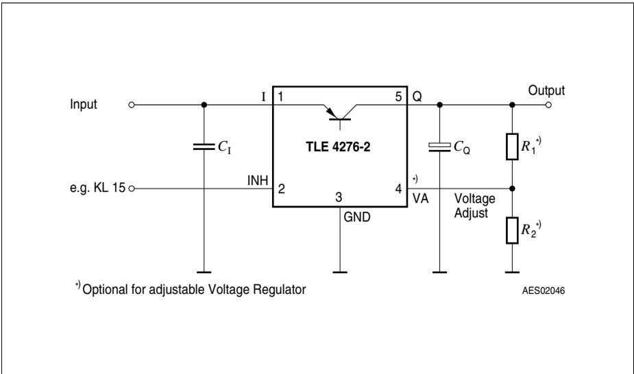
**Figure 4 Application Circuit**
