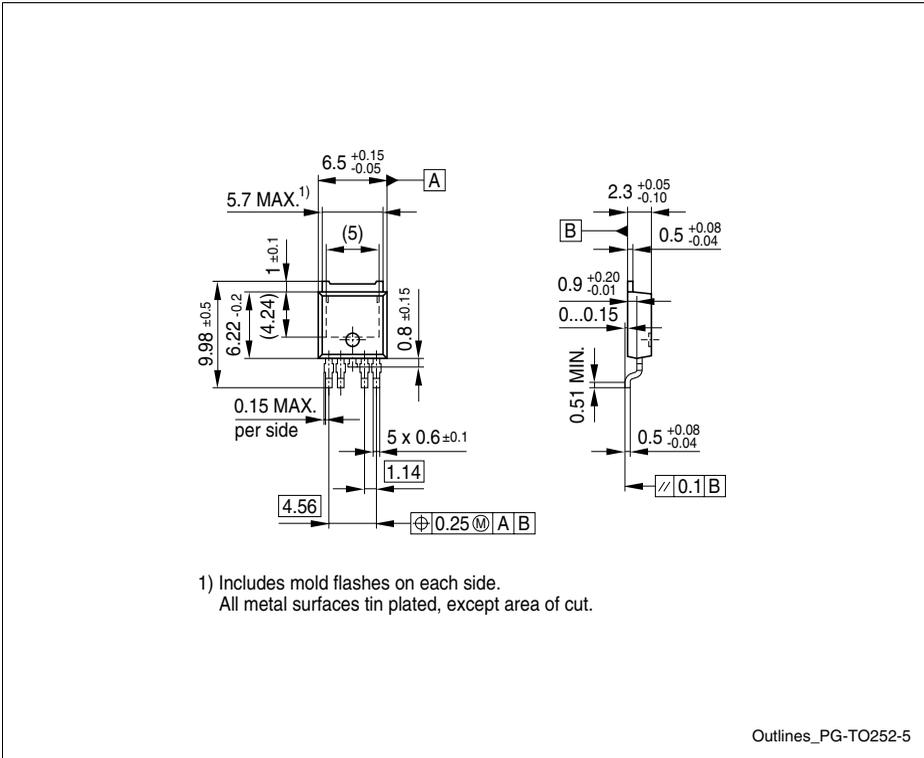
**Figure 7 PG-TO252-5 (Plastic Green Transistor Single Outline)**
