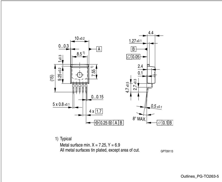
Figure 6 PG-TO263-5 (Plastic Green Transistor Single Outline)
