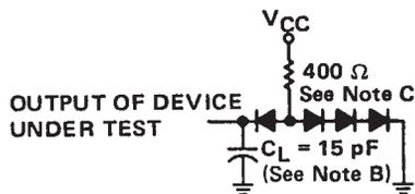
All three outputs are loaded during testing.
