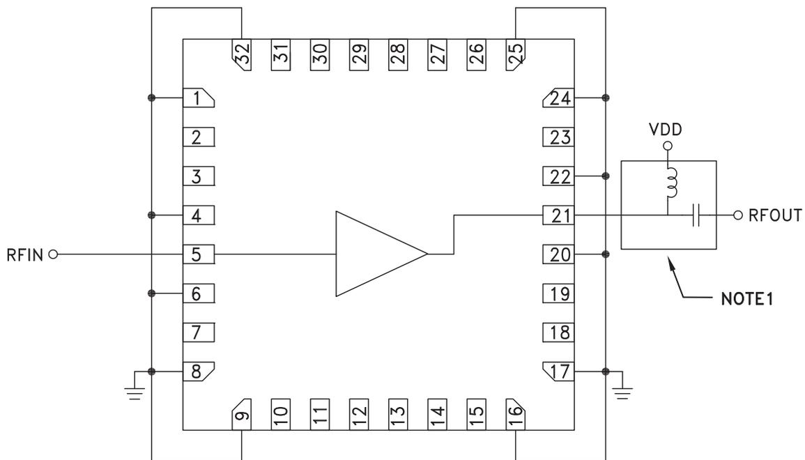
**NOTE 1:** Drain Bias (Vdd) must be applied through a broadband bias tee or external bias network.
