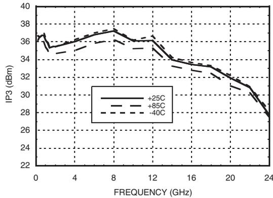
**Output IP3 vs. Vdd @ Pout = 16 dBm / Tone**
