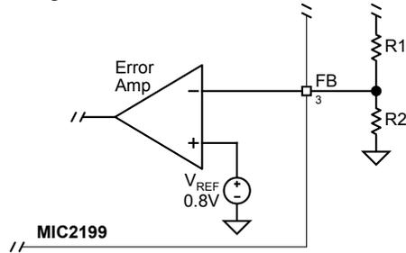
**Figure 6. Voltage-Divider Configuration**
