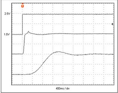
Figure 2. Time-domain response for the Figure 1 circuit, with optimization circuitry (middle trace) and without it (bottom trace).
