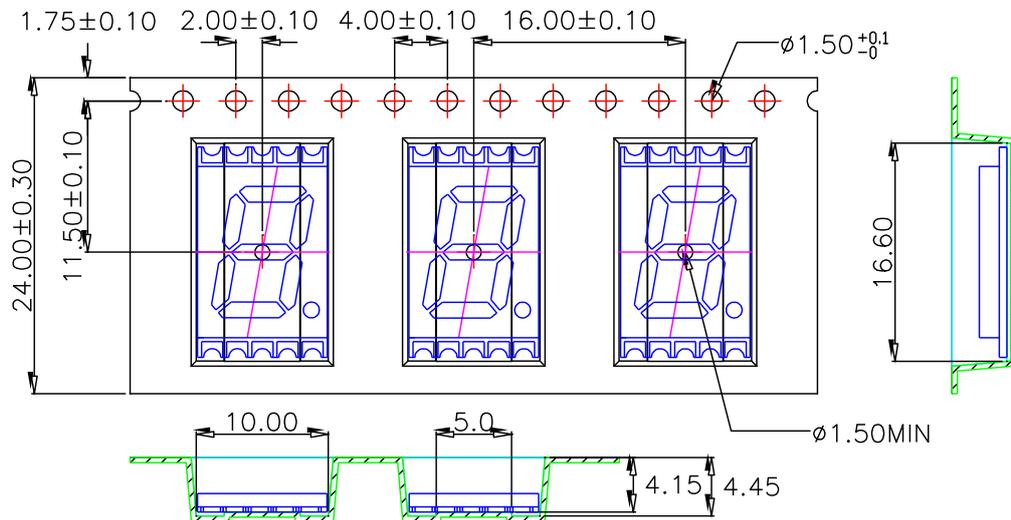
1. 10 sprocket hole pitch cumulative tolerance  $\pm 0.20$ .
