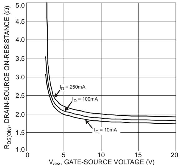
Figure 4 Typical Drain-Source On-Resistance vs. Gate-Source Voltage
