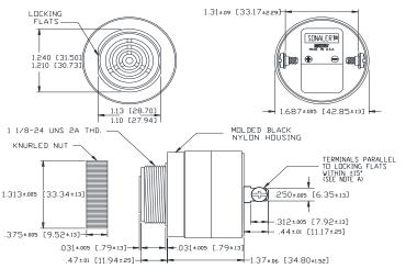
NOTE A: TERMINALS-032 BRASS TIN PLATED, TAPPED FOR #6-32 SCREW. TWO #6-32 NICKEL PLATED BRASS SCREWS INCLUBED. WILL ACCEPT 1/4' QUICK CONNECT.
