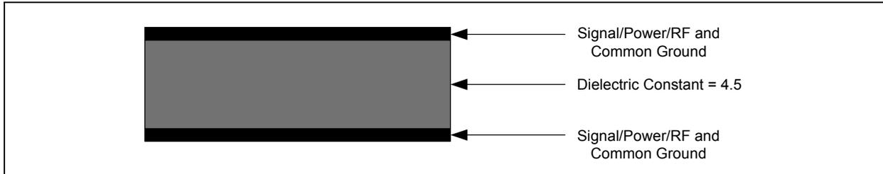
**FIGURE 4-4: FOUR BASIC COPPER FR4 LAYERS**
