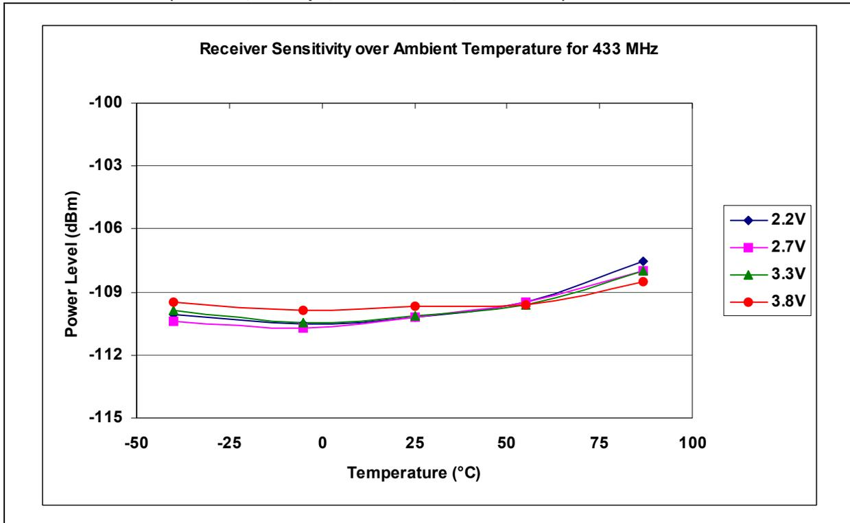
**FIGURE 5-6: RECEIVER SENSITIVITY OVER AMBIENT TEMPERATURE**
