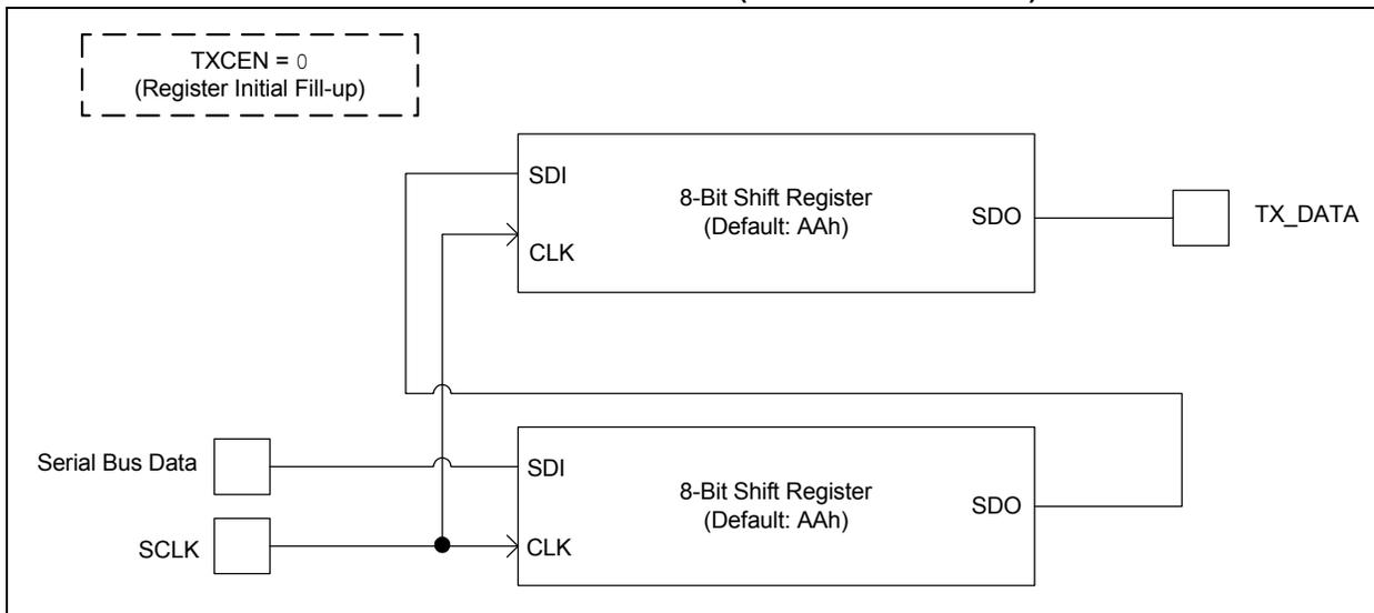
**FIGURE 3-15: TX REGISTER BLOCK DIAGRAM (DURING TRANSMIT)**
