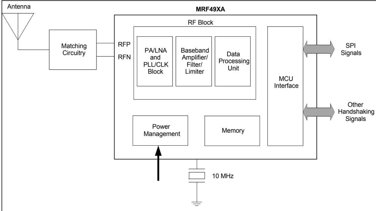
**FIGURE 1-2: MICROCONTROLLER TO MRF49XA INTERFACE**
