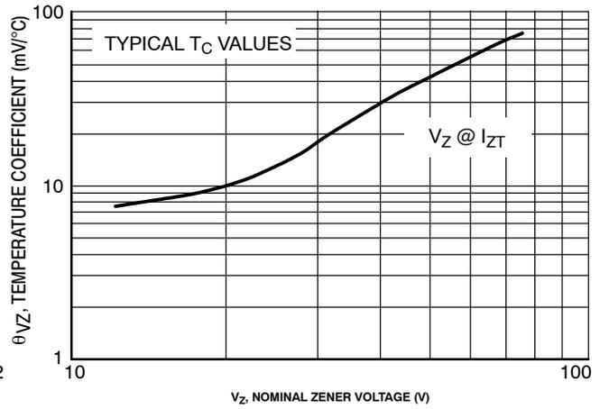
**Figure 2. Temperature Coefficients (Temperature Range -55°C to +150°C)**
