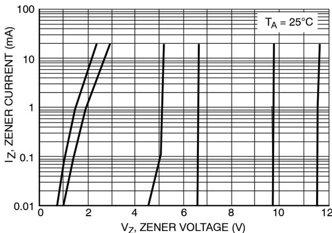
Figure 9. Zener Voltage versus Zener Current (V<sub>Z</sub> Up to 12 V)
