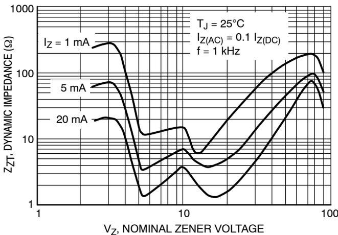
**Figure 5. Effect of Zener Voltage on Zener Impedance**
