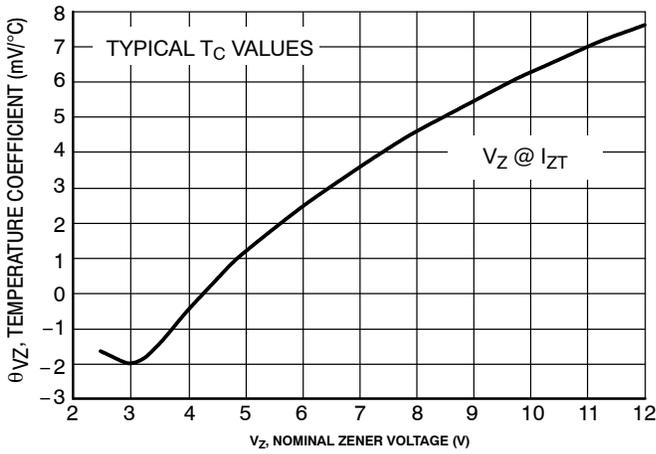
**Figure 1. Temperature Coefficients (Temperature Range -55°C to +150°C)**
