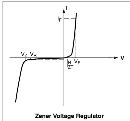
**ELECTRICAL CHARACTERISTICS** ( $T_A = 25^\circ\text{C}$  unless otherwise noted,  $V_F = 0.9\text{ V Max. @ } I_F = 10\text{ mA}$ )
