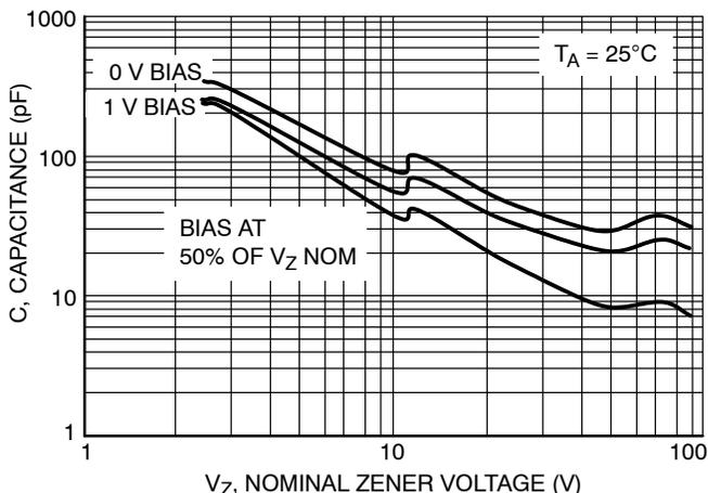
Figure 7. Typical Capacitance
