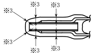
※3 Coating thickness is 0.4mm Min. from the live part.
