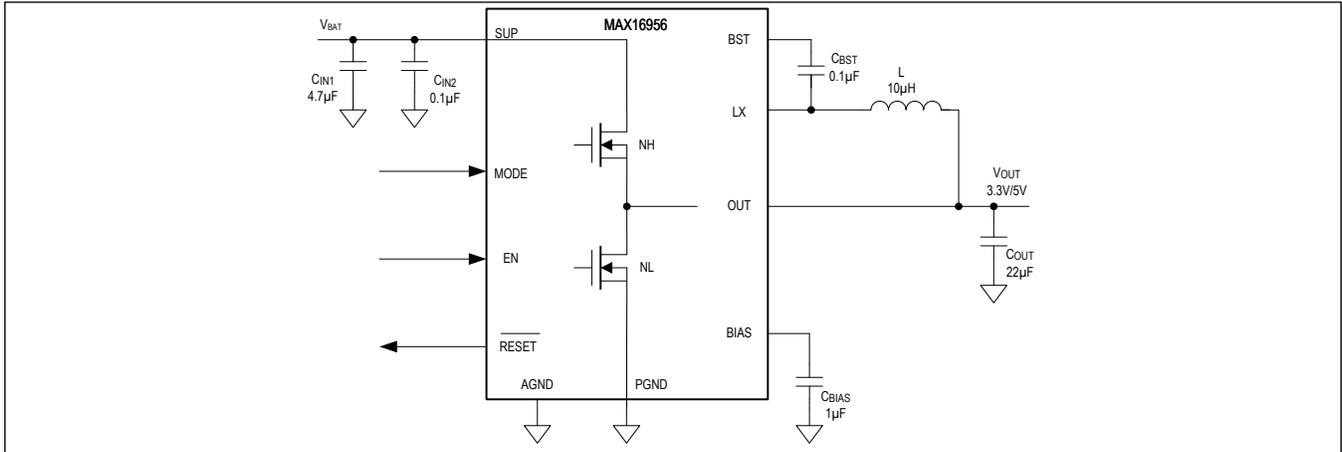
MAX16956AUBC/V+, Variable Output Voltage, 10-Pin µMAX
