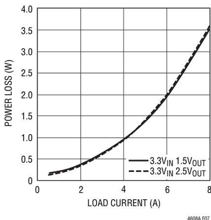
Figure 7. 3.3V<sub>IN</sub>, 2.5V and 1.5V<sub>OUT</sub> Power Loss
