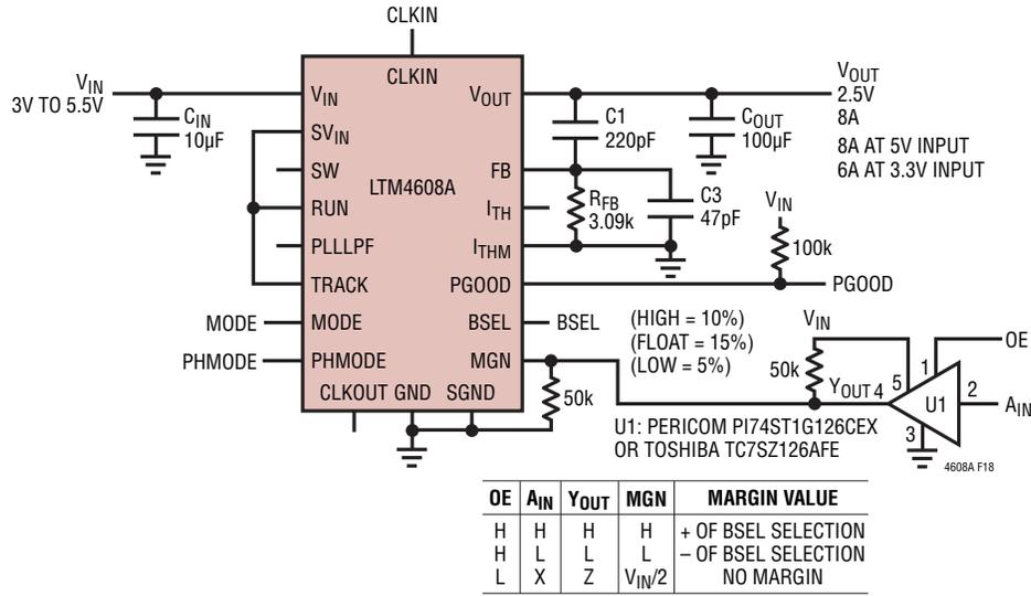
Figure 18. Typical 3V to 5.5V<sub>IN</sub>, 2.5V at 8A Design
