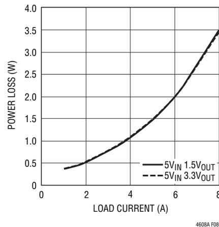
Figure 8. 5V<sub>IN</sub>, 3.3V and 1.5V<sub>OUT</sub> Power Loss
