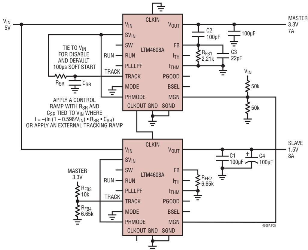
Figure 5. Dual Outputs (3.3V and 1.5V) with Tracking
