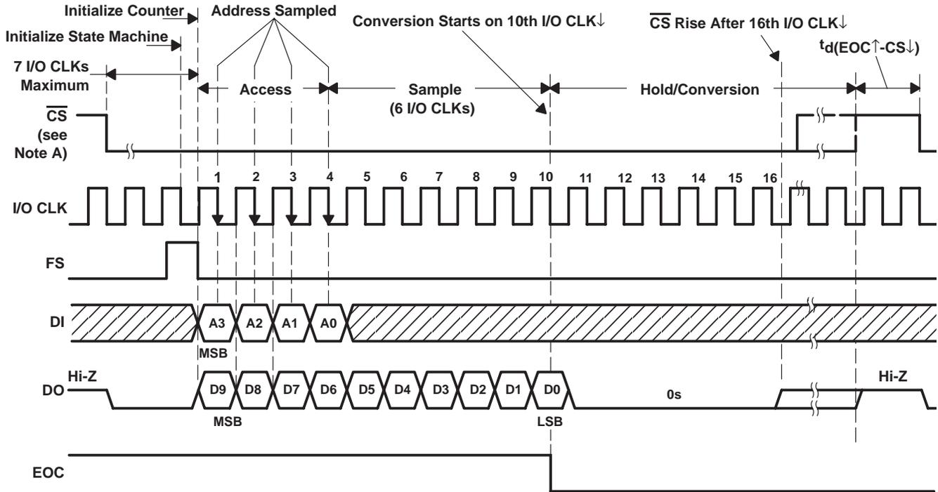
NOTE A: To minimize errors caused by noise at  $\overline{\text{CS}}$ , the internal circuitry waits for a setup time after  $\overline{\text{CS}}\downarrow$  before responding to control input signals. No attempt should be made to clock in input data until the minimum  $\overline{\text{CS}}$  setup time elapses.
