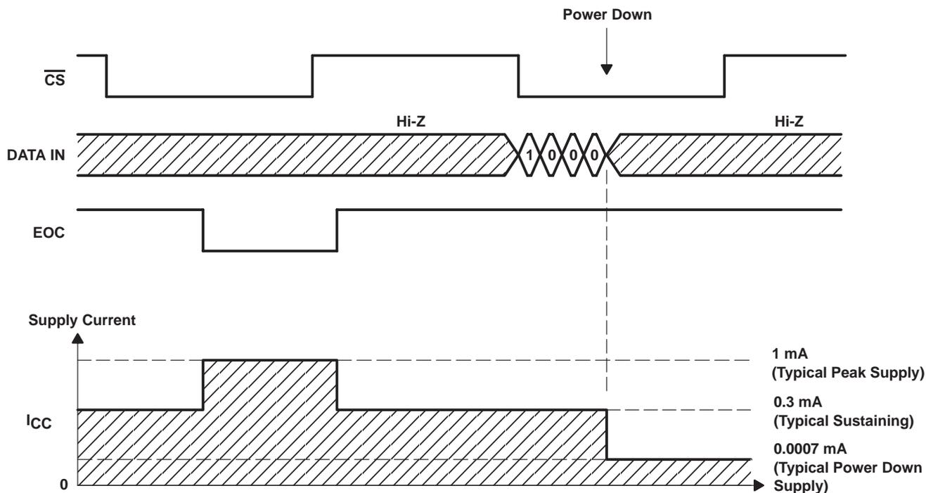
**Figure 3. Typical Supply Current During Conversion/Power Down**
