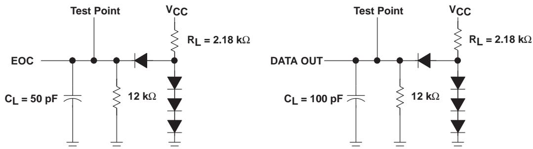
Figure 7. Load Circuits
