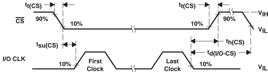
Figure 10. CS and I/O CLK Voltage Waveforms
