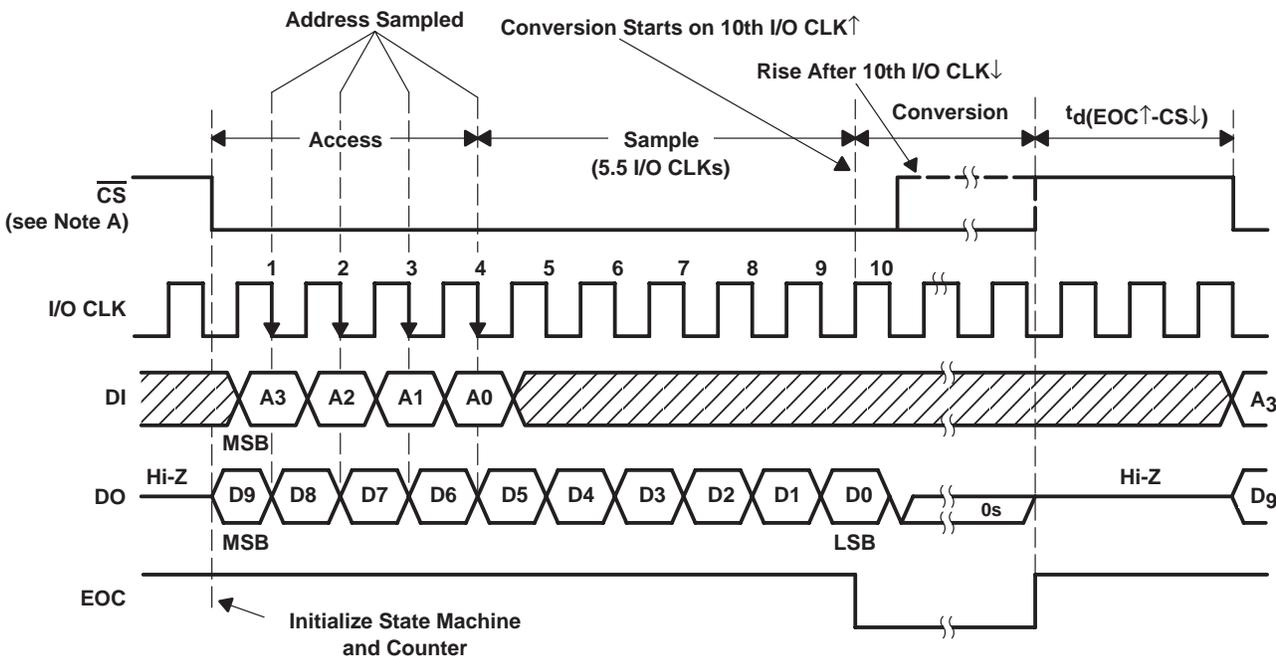
NOTE A: To minimize errors caused by noise at  $\overline{\text{CS}}$ , the internal circuitry waits for a setup time after  $\overline{\text{CS}}\downarrow$  before responding to control input signals. No attempt should be made to clock in input data until the minimum  $\overline{\text{CS}}$  setup time has elapsed.
