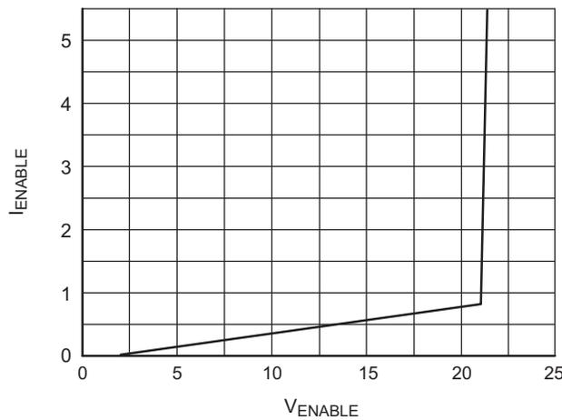
Figure 16. 12 mA ENABLE Current vs. ENABLE Voltage
