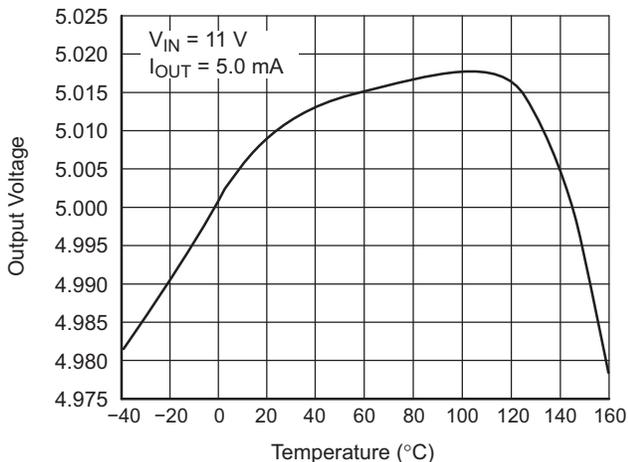
Figure 8. Output Voltage vs. Temperature for  $V_{OUT2}$
