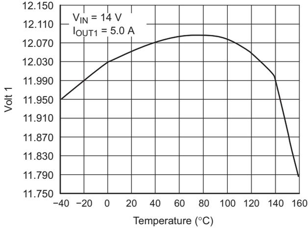
Figure 2. Output Voltage vs. Temperature for  $V_{OUT1}$
