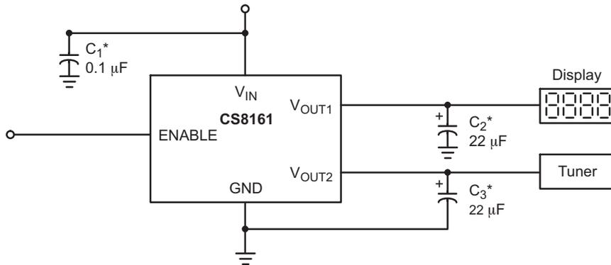
\*  $C_1$  required if regulator is located far from power supply filter.
