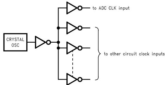
Figure 34. Isolating the ADC Clock from Digital Circuitry
