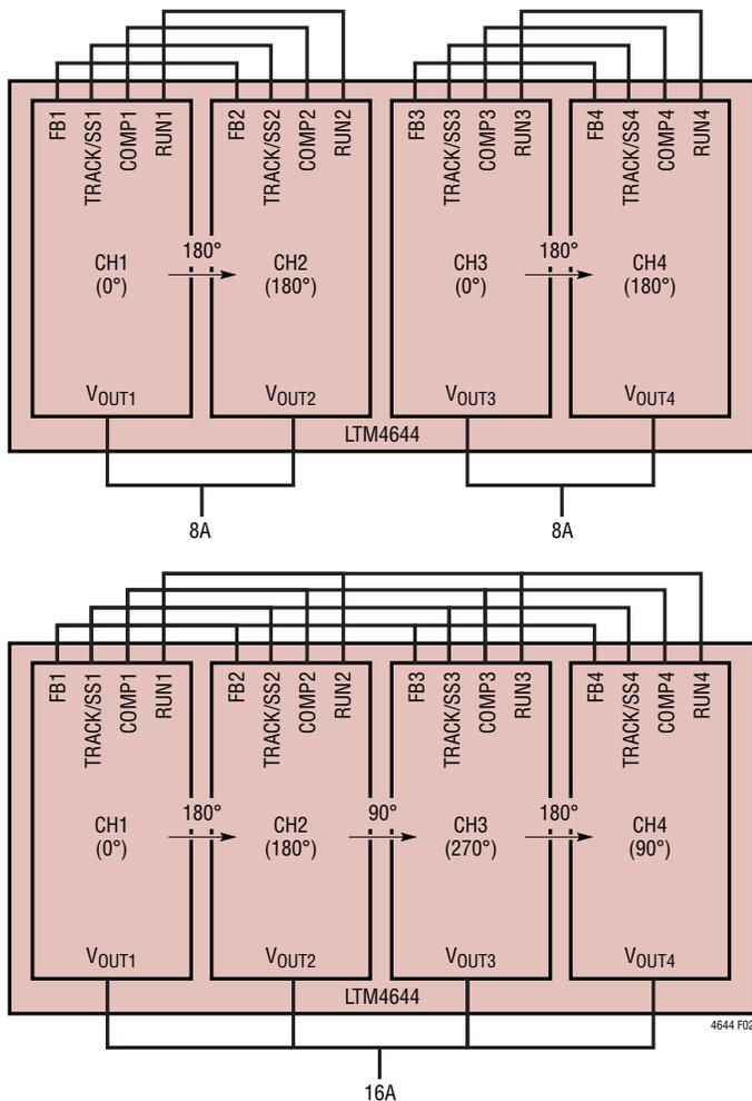
**Figure 2. 2+2 and 4 Channels Parallel Concept Schematic**
