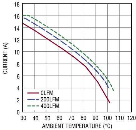
Figure 25. 12V<sub>IN</sub> to 3.3V<sub>OUT</sub>
