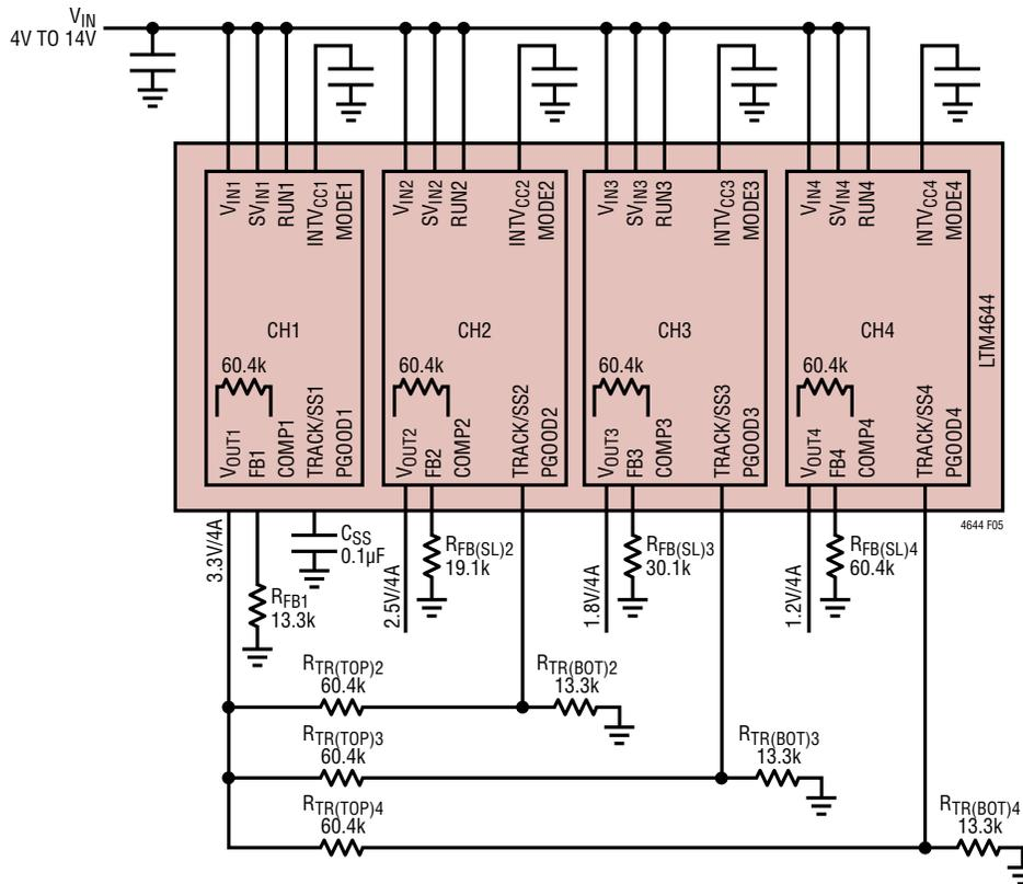
Figure 5. Output Ratiometric Tracking Schematic
