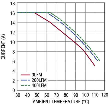
Figure 18. 5V<sub>IN</sub> to 1.0V<sub>OUT</sub> Derating Curve 4-Channel Paralleled, BGA Heat Sink
