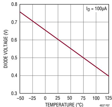
Figure 7. Diode Voltage  $V_D$  vs Temperature  $T(^{\circ}\text{C})$
