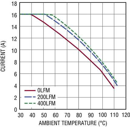
Figure 19. 12V<sub>IN</sub> to 1.0V<sub>OUT</sub> Derating Curve 4-Channel Paralleled, BGA Heat Sink
