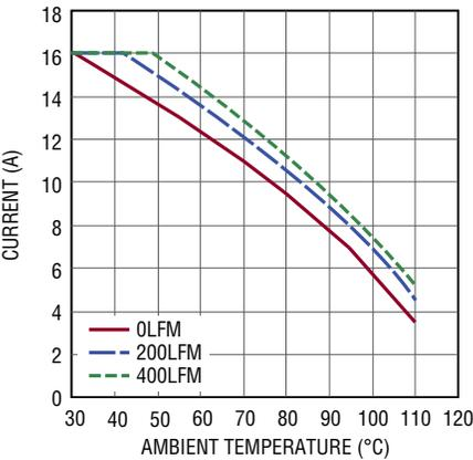
Figure 17. 12V<sub>IN</sub> to 1.0V<sub>OUT</sub> Derating Curve 4-Channel Paralleled, No Heat Sink
