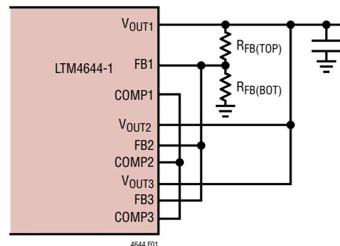
**Figure 1. LTM4644-1 Feedback Resistor for Paralleling Application**
