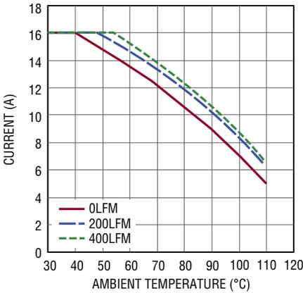
Figure 20. 5V<sub>IN</sub> to 1.5V<sub>OUT</sub> Derating Curve 4-Channel Paralleled, No Heat Sink
