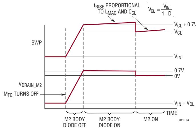
Figure 4. Detail of Region 3 from the Timing Diagram in Figure 2. When  $M_{FG}$  Turns Off in Active Clamp Reset,  $I_{LMAG}$  Initially Slews Up SWP's Voltage from  $V_{IN}$  to  $V_{CL} + 0.7V$ , at Which Point  $M_2$ 's Body Diode Turns On and Allows  $I_{LMAG}$  to Flow into  $C_{CL}$
