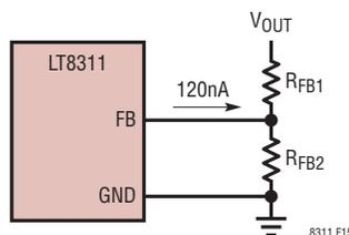
Figure 15. Setting Output Voltage of Forward Converter
