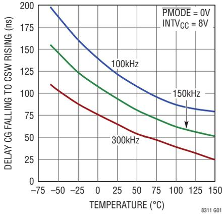
**Jitter in CG Turn-Off Delay to CSW Rising Edge vs CSW Switching Frequency and Junction Temp**
