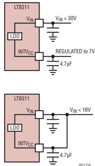
Figure 14. V<sub>IN</sub> and INTV<sub>CC</sub> Pin Configurations
