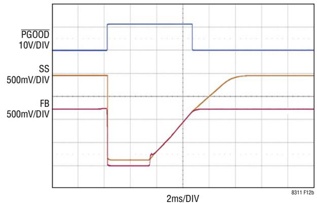
(b) Output Overshoot Control with  $C_{\text{SS}} = 33\text{nF}$ . LT8311  $V_{\text{IN}}$  Powered from a 12V Housekeeping Supply, Which Also Pulls Up on the  $\overline{\text{PGOOD}}$  Pin Through a 100k External Resistor
