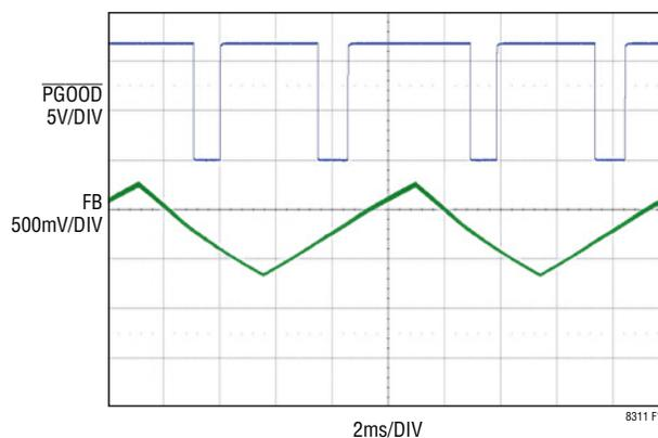
Figure 11. Power Good Activates ( $\overline{\text{PGOOD}} = \text{Low}$ ) When the LT8311's FB Pin Voltage Is Within  $\pm 7\%$  of Its Regulated Target (1.227V). The  $\overline{\text{PGOOD}}$  Pin Is Pulled Up Externally to a 12V Housekeeping Supply Through a 100k External Resistor
