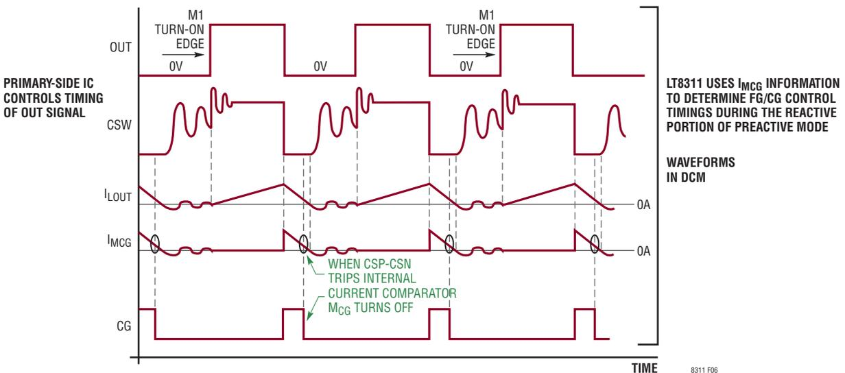
Figure 6. During the Reactive Portion of Preactive Mode, the LT8311 Turns Off  $M_{CG}$  When the Current in  $M_{CG}$ ,  $I_{MCG}$ , Trips the LT8311's Internal Current Comparator. The Inputs to the Comparator Are CSP and CSN and the Current Sense Trip Voltage Is Programmed by Choosing Appropriate CSP/CSN Series Resistors
