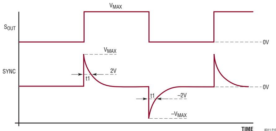
**Figure 19. Positive and Negative SYNC Edges Are Generated on the Rising and Falling Edges of S<sub>OUT</sub>, Respectively. The LT8311 Requires Pulse Width Time, t<sub>1</sub>, to Be at Least 50ns (Typical) with the SYNC Pin Voltage at ±2V (or Greater Overdrive) to Trip the Internal SYNC Detect Comparators.**
