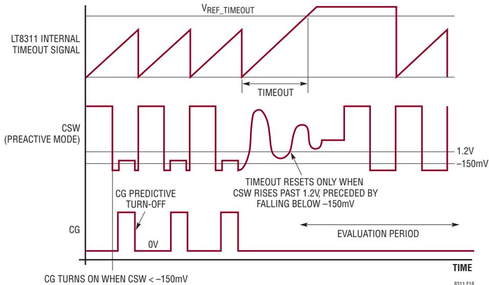
**Figure 18. If Timeout Is Triggered in Preactive Mode, LT8311 Shuts Down All Synchronous Conduction and Starts the Evaluation Period (Note: CSW's ringing waveform is caused by the inductor current getting to 0A.)**
