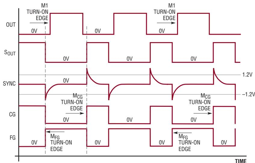
Figure 7. In SYNC Mode, the Primary Side IC Sends  $S_{OUT}$  Signals Through a Pulse Transformer to the LT8311's SYNC Pin.  $SYNC < 1.2V$  Turns on  $M_{FG}$  and Turns Off  $M_{CG}$ .  $SYNC > 1.2V$  Turns On  $M_{CG}$  and Turns Off  $M_{FG}$
