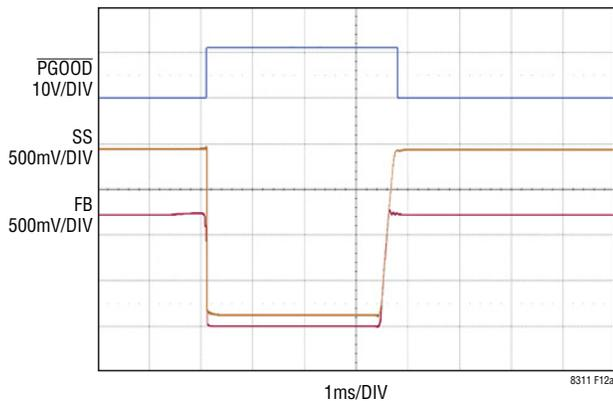
(a) Output Overshoot Control with  $C_{\text{SS}} = 1\text{nF}$ . LT8311  $V_{\text{IN}}$  Powered from a 12V Housekeeping Supply, Which Also Pulls Up on the  $\overline{\text{PGOOD}}$  Pin Through a 100k External Resistor
